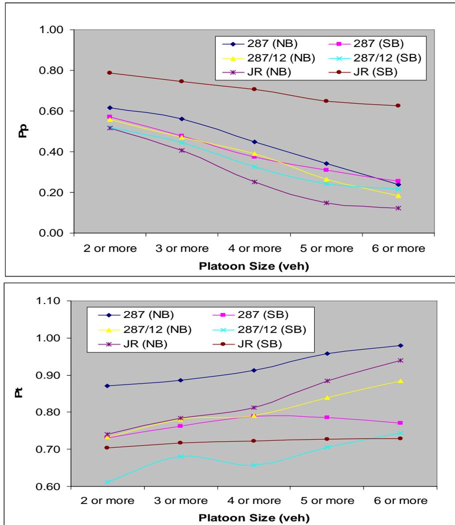
Figure 19  $P_p$  and  $P_t$  versus Platoon Size using Probabilistic Method
