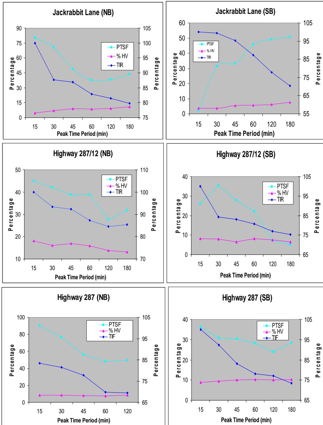
Figure 12 Heavy vehicle, TIF, and PTSF versus Time for Weighted Average Approach
