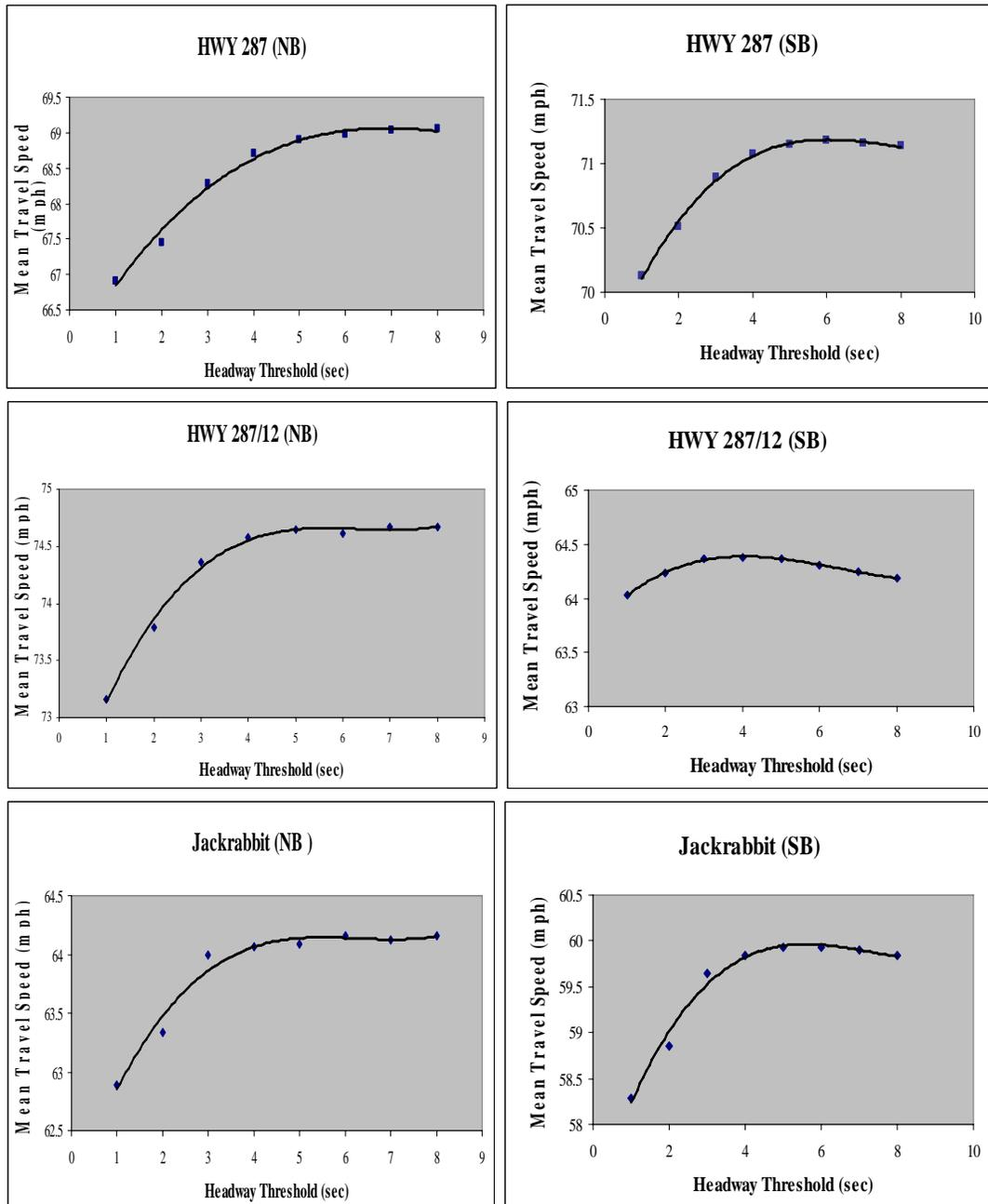
Figure 10 Speed versus Headway Threshold Value (sec)
