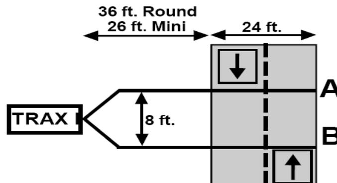
Figure 9 Road Tube Layout for Data Collection (Courtesy of Jamar Technologies, Inc. )
