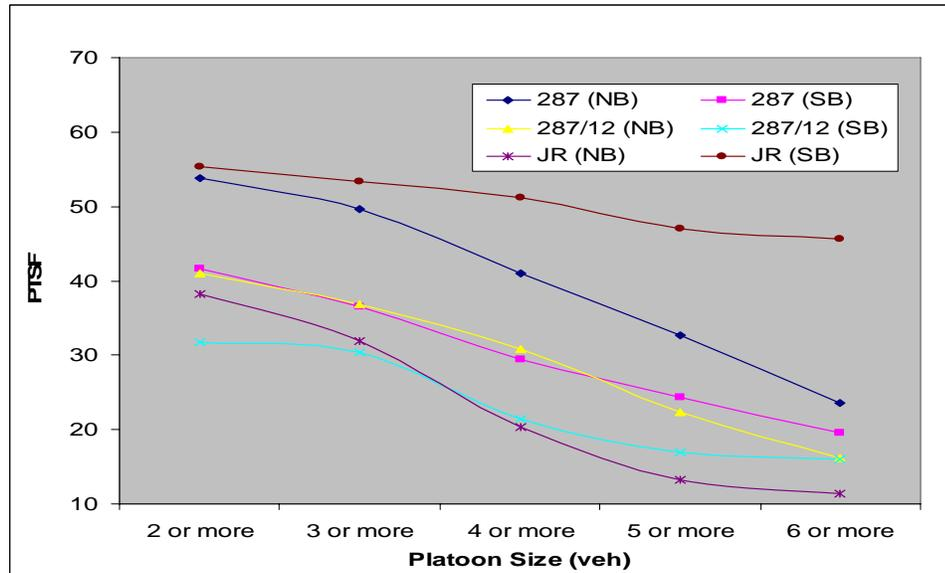
Figure 18 PTSF versus Platoon Size using Probabilistic Method
