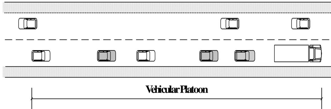
Figure 6 A Vehicular Platoon Behind a Truck on a Two-Lane Highway
