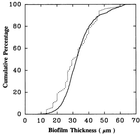
FIG. 1. Biofilm thickness (---) and tracer particle (—) spatial distributions.
