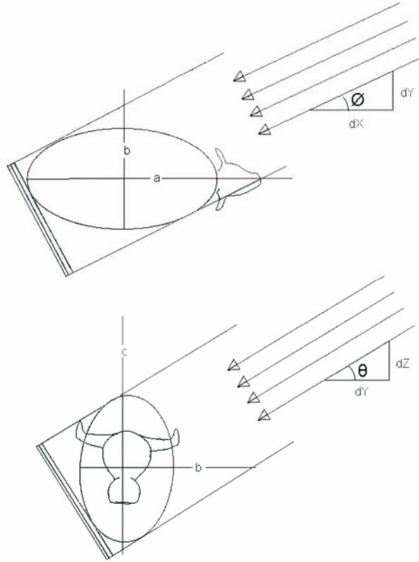
Fig. 2.1. View factors on horizontal x-y axis (top) and vertical y-z axis (bottom) used to estimate view factor of an ellipsoid ( $a \neq b \neq c$ ).
