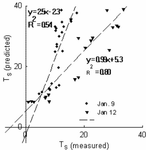
Fig 5.3. Measured (Infra-red thermometer) and predicted (RadTherm) surface temperatures for two days on January 2004.
