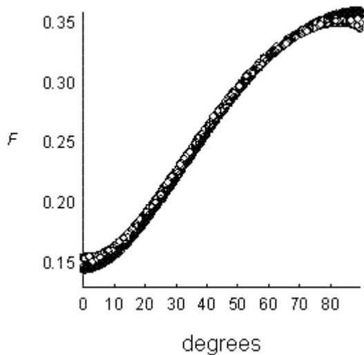
Fig. 2.2. View factor ( $F$ ) of an ellipsoid at different orientations to the azimuth ( $\theta$ ):  $\circ$  mid-day observations ( $\theta > 14.65^\circ$ ),  $\bullet$  morning and afternoon observations ( $\theta < 14.65^\circ$ ).
