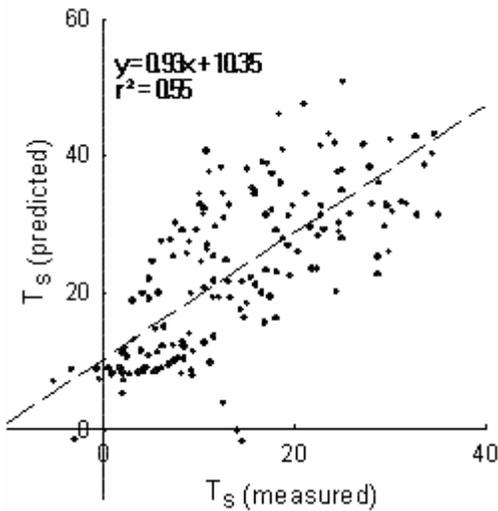
Fig. 5.2. Measured (Infra-red thermometer) and predicted (RadTherm) surface temperatures for January 2004.
