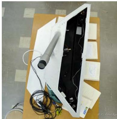
Figure 1. Montana State University “Dark Star” Spectrograph
