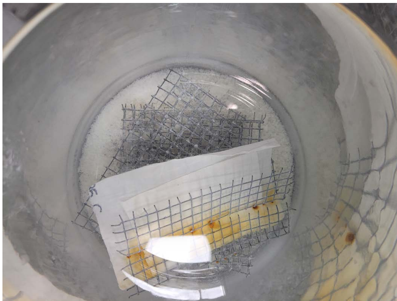
Figure 5.10: Oxidation of stainless steel cage on HB-212 in distilled water with matrix material covering bottom of jar.
