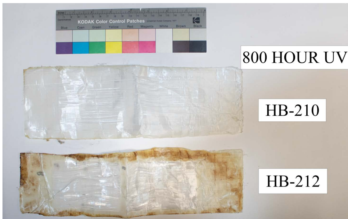
Figure 6.2: UV aging of HB-210 and HB-212 after 800 hours.
