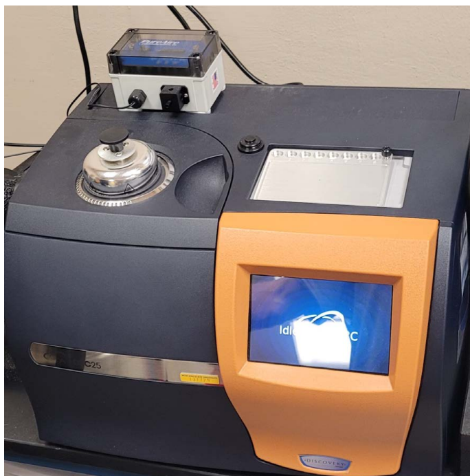
Figure 3.7: TA Differential Scanning Calorimetry Machine (DSC 25).
