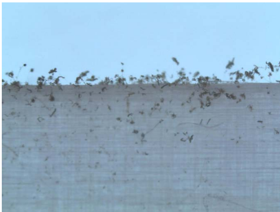
Figure 5.11: Trace fungal growth, 28 days after fungal inoculation on single layer SR-5241.
