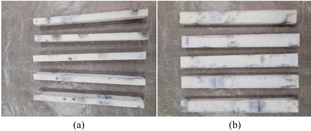
Figure 5.1: Beginning stages of fungal growth on HB-212 salt water pressed panels.
