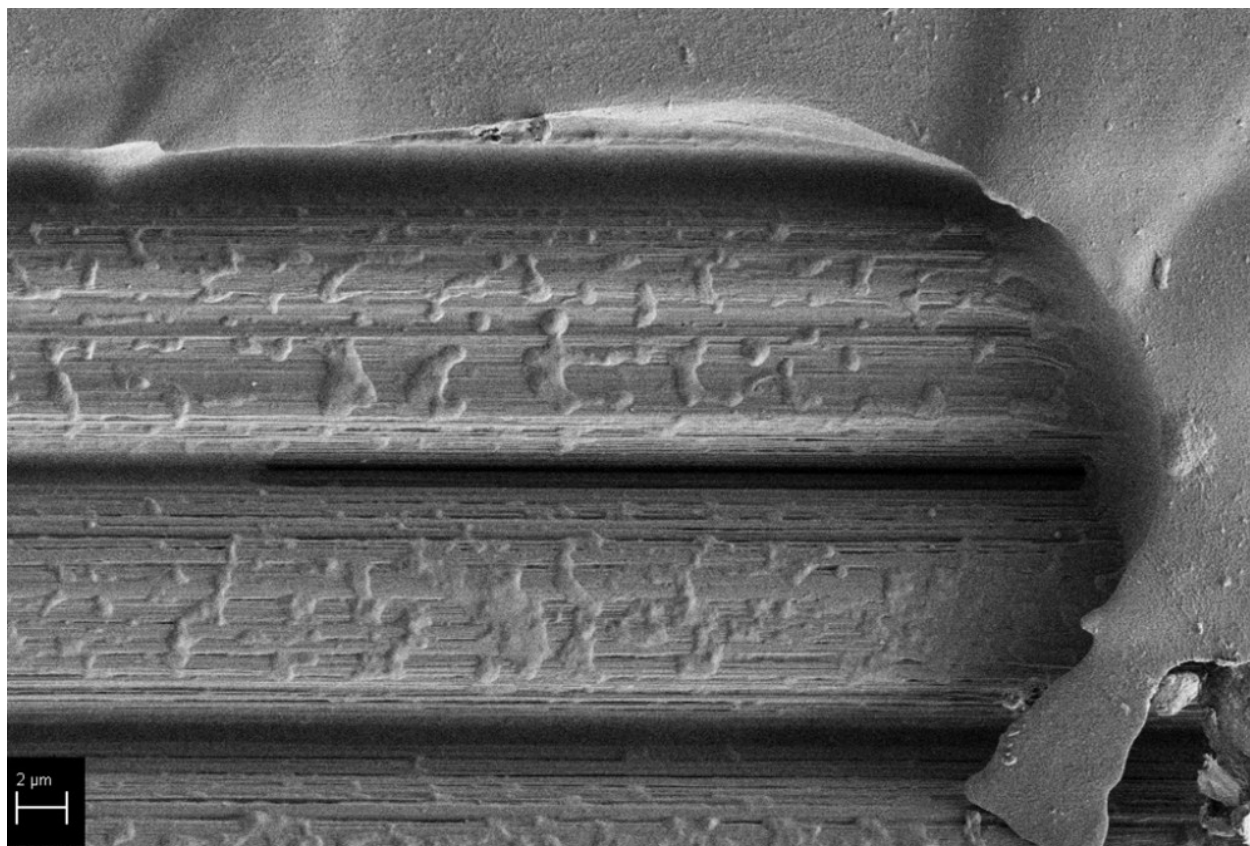
Figure 5.19: Enlarged SEM view of unaged HB-210 with matrix voids exposing fibers on the surface.
