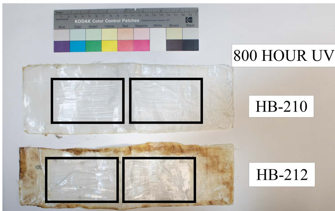
Figure 6.3: Bare fibers exposed in the UV window highlighted black after 800 hours exposure.
