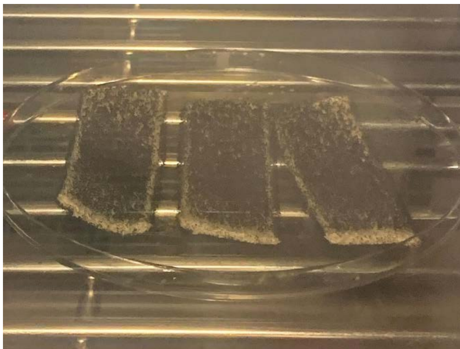
Figure 5.5: NTS control samples 7 days after inoculation.
