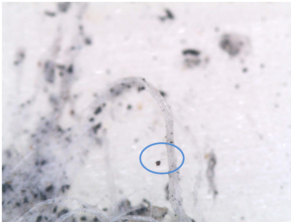
Overview of Dyneema HB-212, Post 28 Days – 50x Magnification Fungal growth observed on frayed edge
