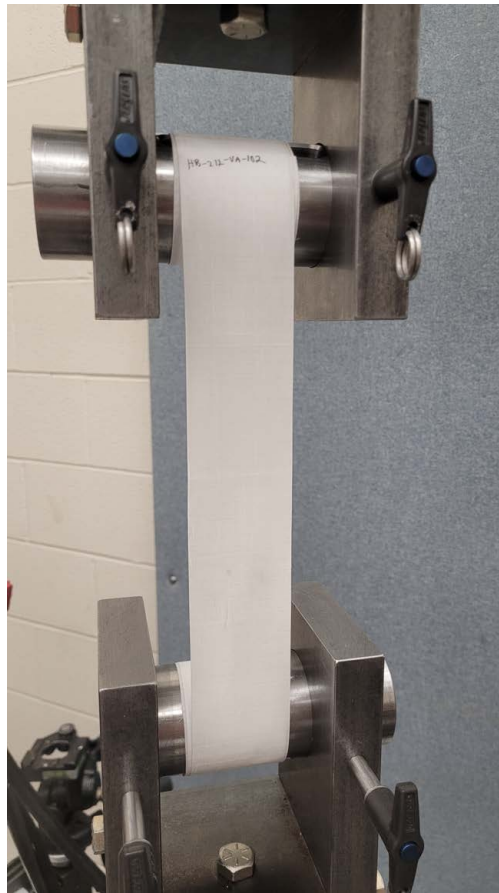
Figure 4.1: Unaged tensile coupon mounted on capstan grips, 30 cm center to center length.
