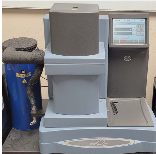
Figure 3.9: TA Q800 Dynamic Mechanical Analysis machine.
