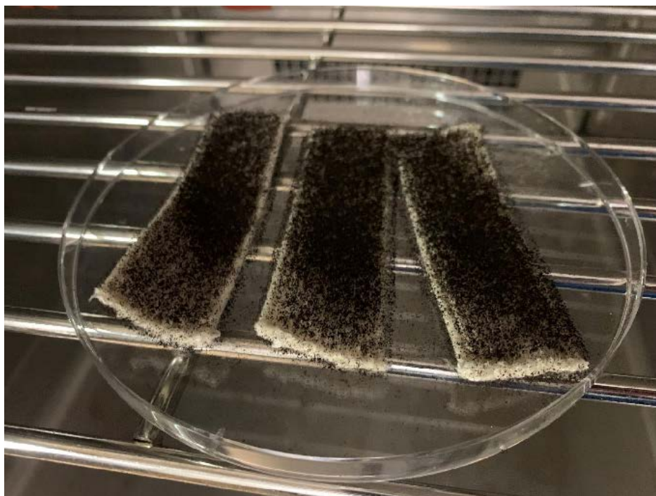
Figure 5.6: NTS control samples 28 days after inoculation.
