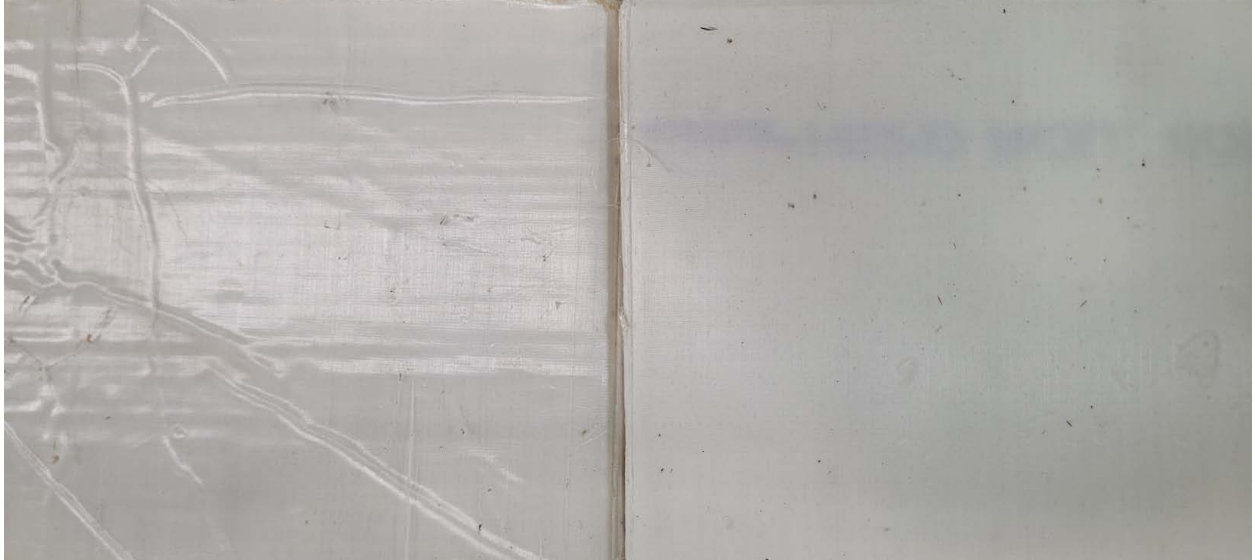
Figure 3.4: Surface finish comparison of plate consolidation manufacturing methods.
