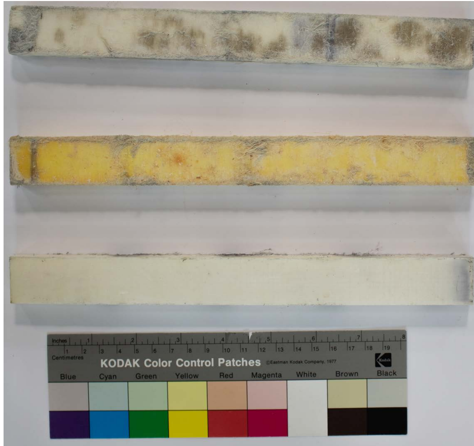
Figure 5.3: 95 layer pressed panel HB-212 samples from top to bottom: salt water, distilled water, and unaged.
