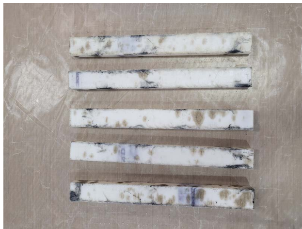
Figure 5.2: Interlaminar fungal growth after 669 days in salt water.
