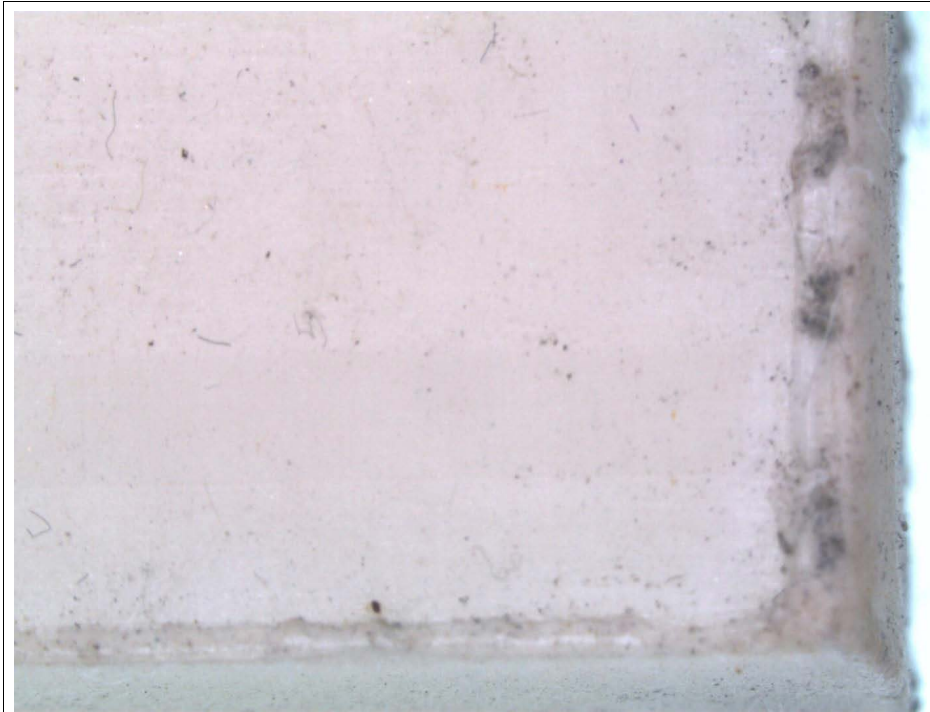
Overview of Dyneema HB-212, Post 28 Days – 8x Magnification
