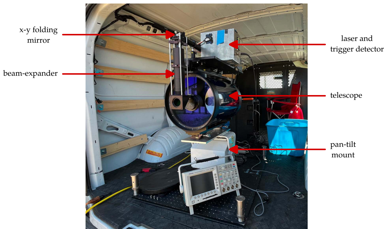
Figure 3. Picture of the lidar system during data collection.
