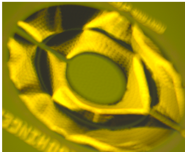
Figure 29: A burst membrane due to trapped evolved hydrogen gas.
