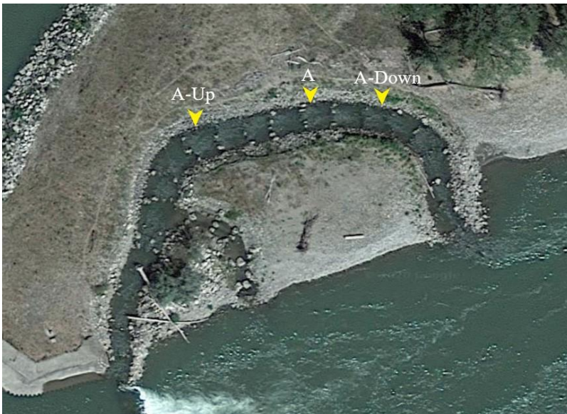
Figure 6. Water surface elevation locations used for slope-area flow rate calculations (Google Earth, 2020).
