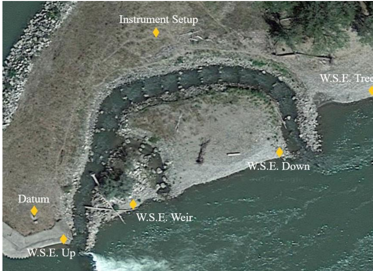
Figure 4. Approximate locations of water surface elevation survey points and associated datum and setup locations (Google Earth, 2020).
