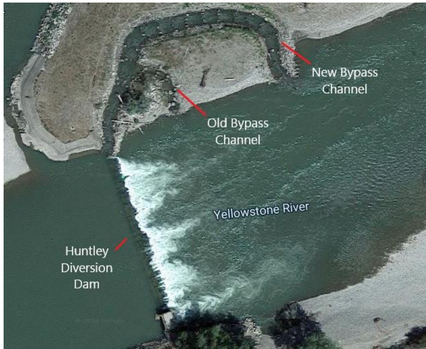
Figure 2. Huntley Diversion and old and new nature-like bypass channels. Image from Google Earth (2020).
