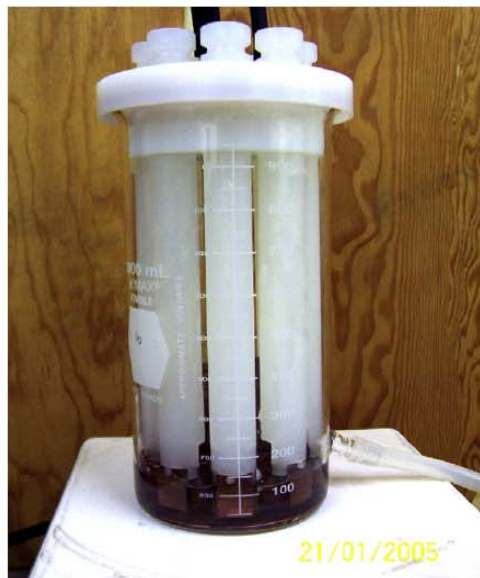
Fig. 1 – Modified CDC reactor showing the paired copper coupons (1.5 × 1.7 cm inside, 1.5 × 1.3 cm outside on the rods), base plate (bottom of the reactor) and the blade in the center.
