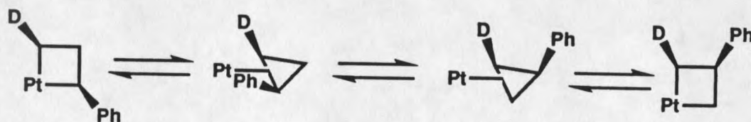
Figure 24. Proposed mechanism of Puddephatt rearrangement.
