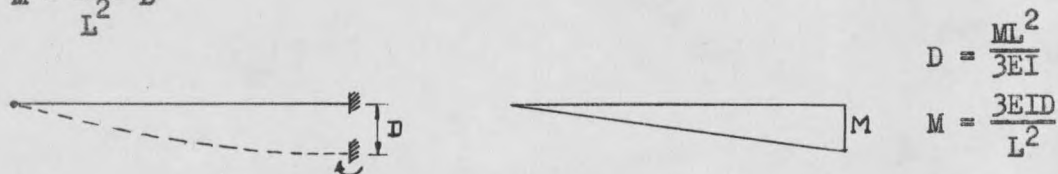
Fig. 3b Conjugate beam relations--far end pin-connected.
