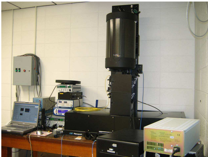
Figure 5.9: A picture of the DIAL instrument in its operational form inside the roofport room of Cobleigh Hall.
