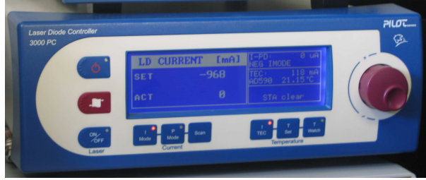
Figure 5.4: A picture of the Sacher Lasertechnik Pilot driver used to control the cascaded tapered amplifier in the vertical DIAL experiments.
