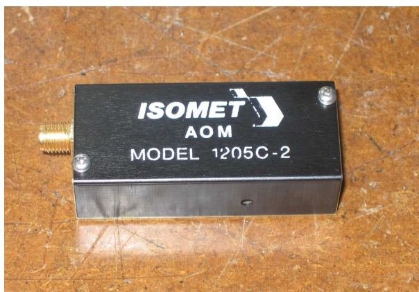
Figure 3.11: A picture of the acousto-optic modulator (AOM) used to pulse the cw laser beam. The entrance aperture is visible on the side, below the “5” in 1205C-2.
