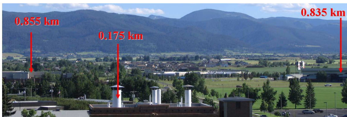
Figure 3.20: A picture of the three hard targets and their ranges used in the horizontal tuning experiments, taken from the roof of Cobleigh Hall at Montana State University, just above the roofport room where the measurements were made.
