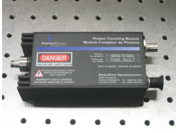
Figure 3.18: A picture of the avalanche photodiode (APD) detector.
