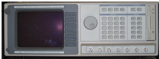
Figure 3.19: A picture of the Stanford Research Systems Multi-channel Scalar (MCS) with display screen used in the horizontal tuning experiments.
