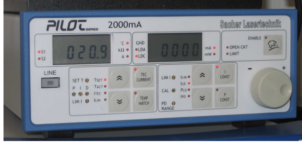
Figure 3.7: A picture of the Sacher Lasertechnik Pilot driver used to control the tapered amplifier in the horizontal tuning experiments.
