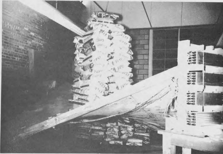
Figure 13. Concentrated Load At The Shell Center.
