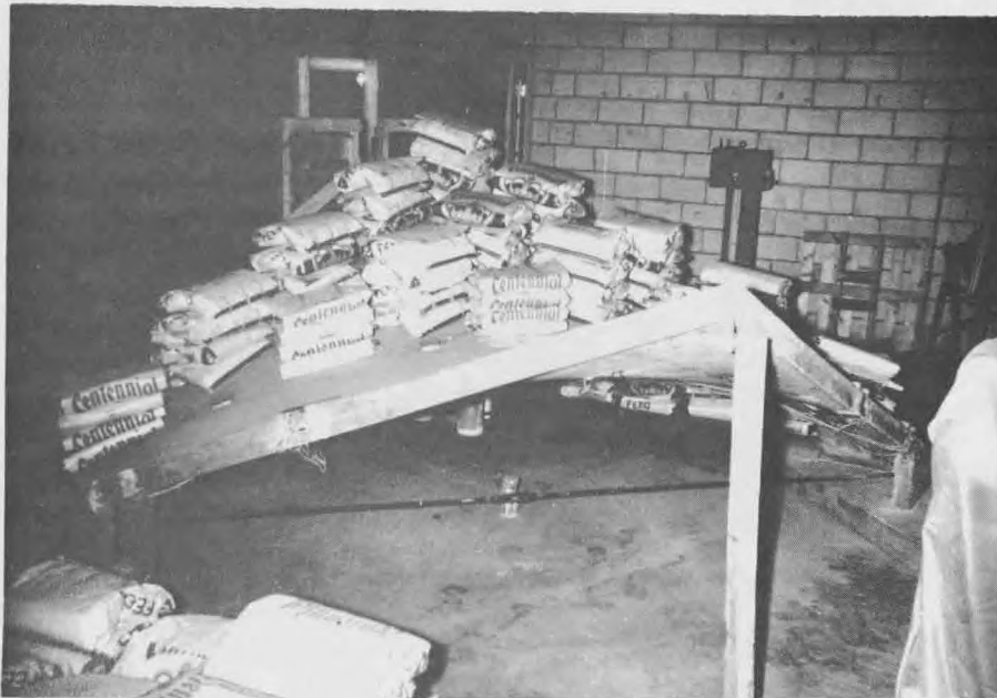
Figure 14. Uniform Load Over Half The Surface Area.
