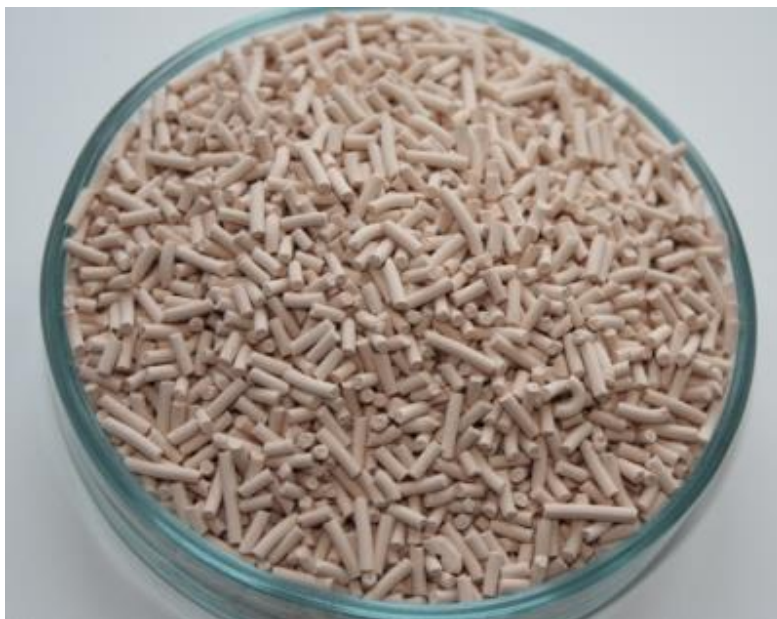
Figure 10: Synthetic zeolite pressed into pellets for industrial use. 94
