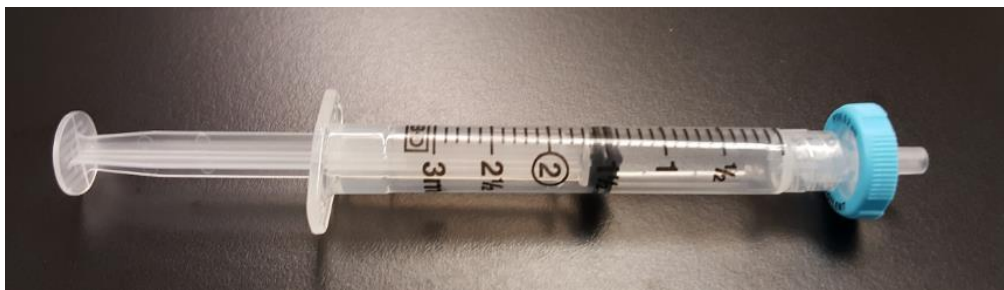
Figure 20: Syringes with 0.2 \mu M filters were used to filter all samples and standards.
