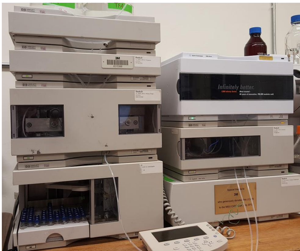
Figure 17: HPLC with RID and DAD used for analysis of all experiments.
