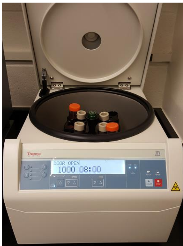
Figure 16: Centrifuge used to separate solid catalyst from solvent following reaction.
