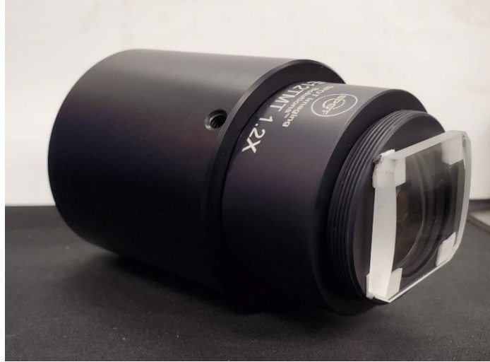
Figure 3.3. The cylindrical lens attached to the microscope adaptor.
