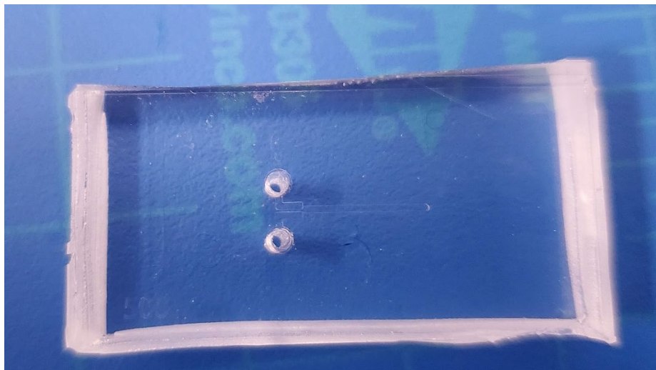
Figure 3.14. A complete microchannel fabricated from PDMS with inlet and outlet ports punched.
