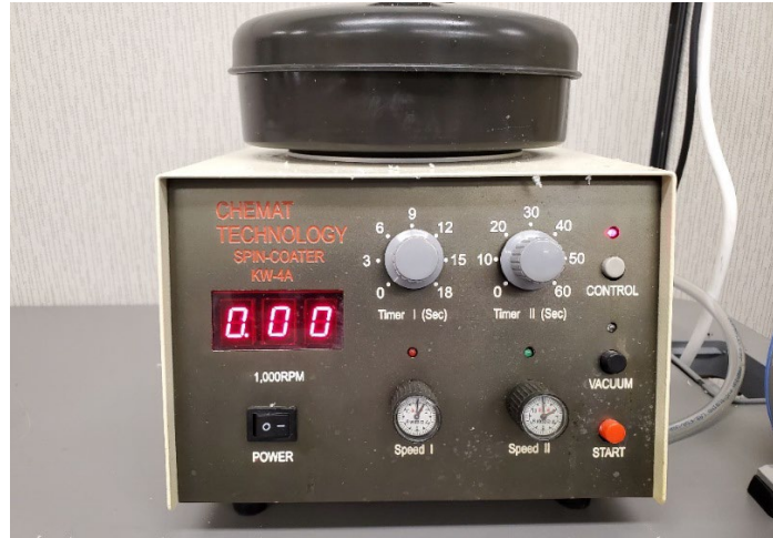
Figure 3.16. The Chemat Technology spin coater used to spin coat the PDMS membrane
