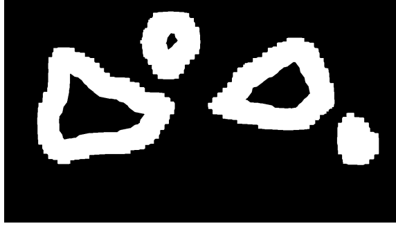
Figure 3.14: M_u , the result of subtracting the matrix of known background areas from the matrix of known foreground areas. the white areas (values of 255) represent the unknown areas between salient and non-salient (background) regions.
