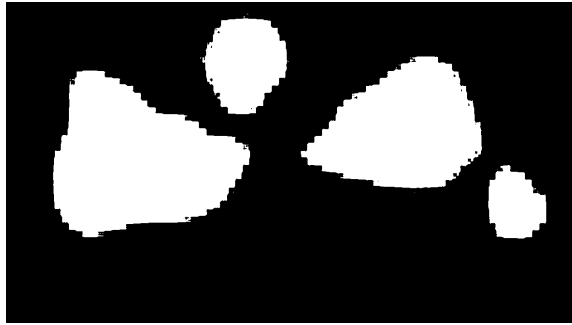
Figure 3.8: The result of applying Otsu Thresholding to the saliency map. White areas (having a value of 255) represent areas of saliency.
