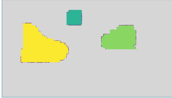
Figure 3.16: M_w , the result of the watershed algorithm. The grey region is non-salient background, and each of the colored regions is a distinct salient region.
