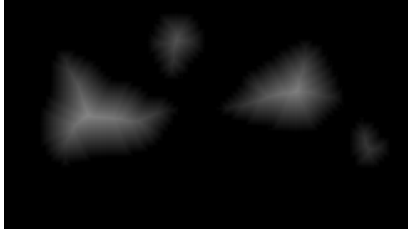
Figure 3.12: Distance transformation D : the center points of the salient regions are exactly white (255), as they are the farthest from a non-salient (black) pixel.
