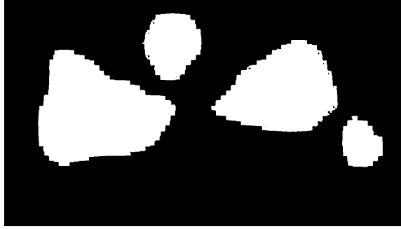
Figure 3.10: The results of the morphological closing step; as the particular saliency map does not have any non-salient holes within a salient region the process had no visible effect.
