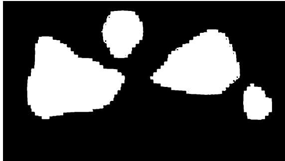
Figure 3.9: The saliency map after applying both Otsu Thresholding and morphological opening. While difficult to see at a small scale, several spots of white noise were removed.
