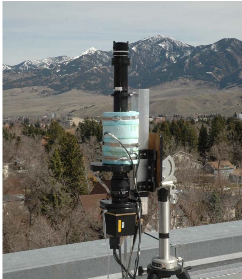
Figure 1.1. The visible-wavelength imaging polarimeter designed in this project, shown operating in full-sky mode.
