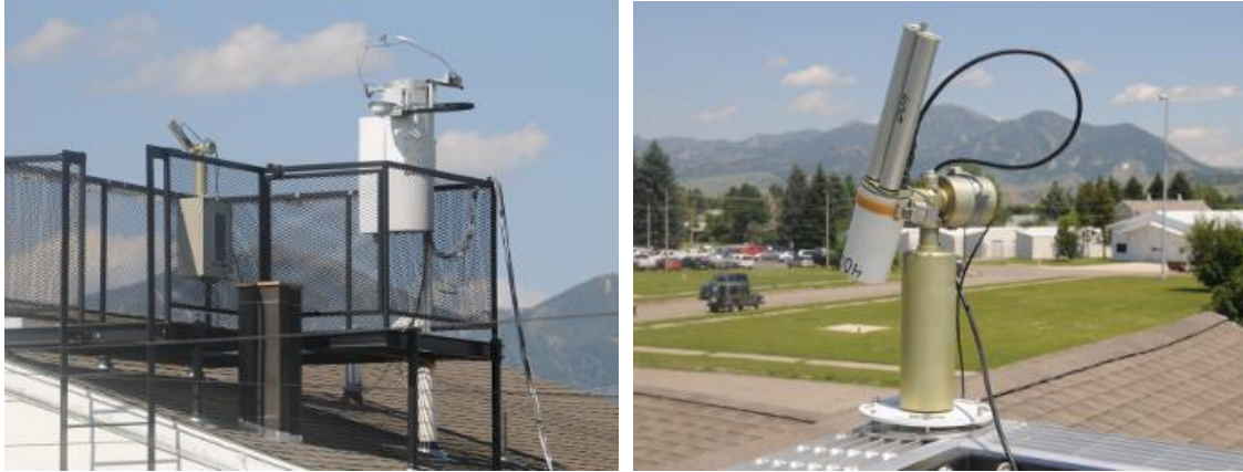
Figure 3. CIMEL solar radiometer located in Bozeman, Montana used by AERONET to retrieve atmospheric data products. The left-hand photo also shows the all-sky polarization imager (photos by Joseph A. Shaw).
