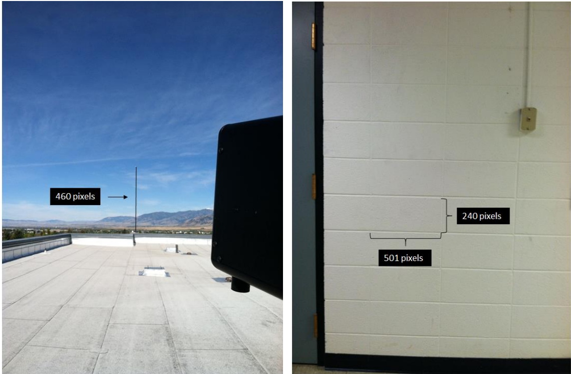
Figure 28. Both images were taken with the same un-zoomed iPhone. (Left) Polarimeter line of sight. The black line indicates the number of pixels (460) from the horizon reference point to the airplane in the sky. (Right) Reference image: used to determine the plane's elevation angle. The average brick was found to be 501 pixels by 240 pixels (0.39 m by 0.19 m). The image was taken 1.65 m away from the wall. The degree-to-pixel ratio was determined to be 3.3^\circ per 120 pixels.
