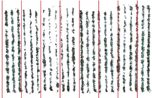
Figure A4.1: Example of how automated plot layouts can cause frameshift. (A) The correctly designated plots account for varying plot spacing to maintain accurate delineation. (B) Automated plot boundaries based on a single plot size and spacing metric lose accuracy across plots.
