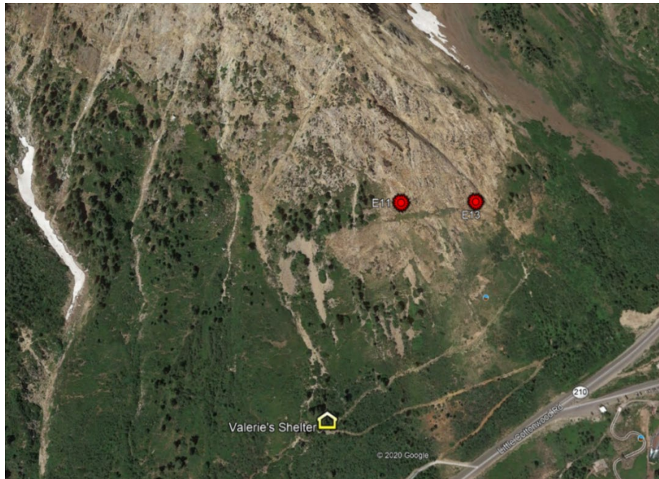
Figure 36 The two 0.8 m 3 Gazex installations proposed for baseline testing in Phase 2 of the testing plan (40°35'6.38"N 111°39'33.81"W).
