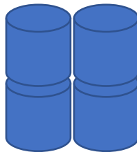
Figure 61 An illustration of the orientation of the four 1 kg cast Pentolite charges assembled to approximate the mortar charge from an Avalanche Guard System
