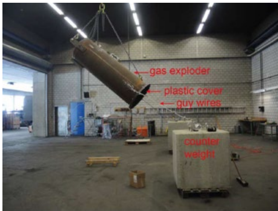
Figure 15 Prototype Gazex system utilized by Simioni (Simioni, 2017).
