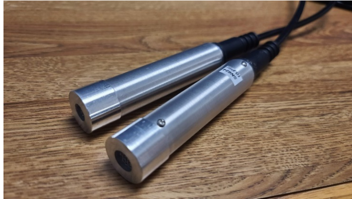
Figure 24 The 10 psi Larcor microphones used for this research.
