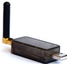
Figure 27 Ronoth LoStik used to provide radio-based communication to and from the DAQs.
