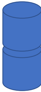
Figure 56 An illustration of the orientation of the two 5 lb cast Pentolite charges assembled to approximate a Pentolite-based Wyssen Tower charge
