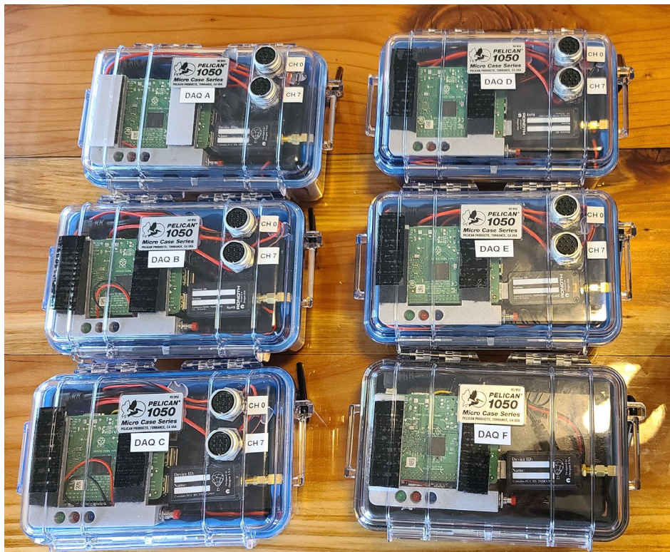
Figure 26 The fleet of 5 operational DAQs constructed for this project (DAQ A - DAQ E), plus an additional DAQ (DAQ F) constructed as a backup unit.
