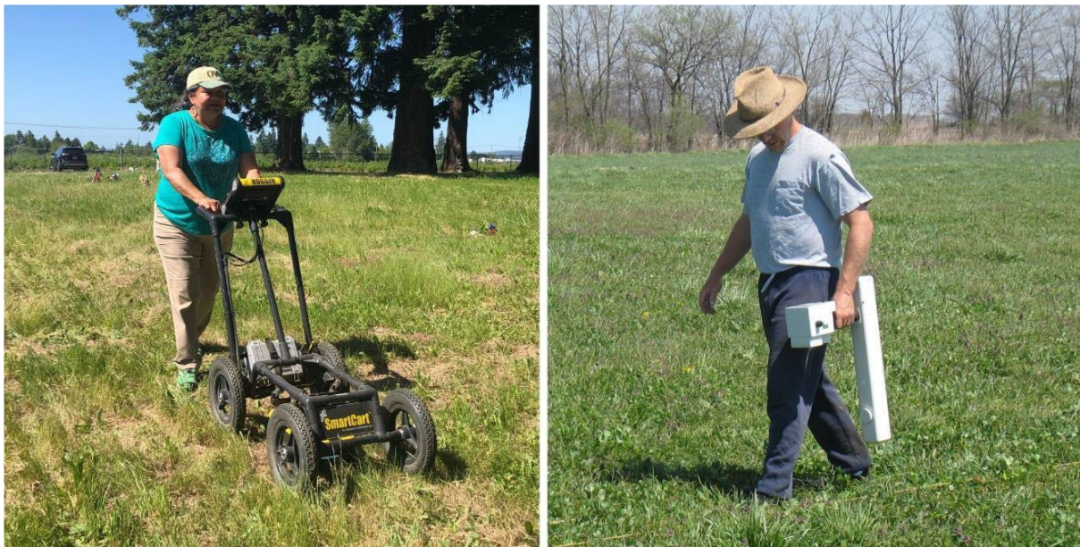
Figure 4.10. The geophysical survey instruments used in the cemetery survey. On the left is an example of ground-penetrating radar, and on the right is an example of a magnetometer.
