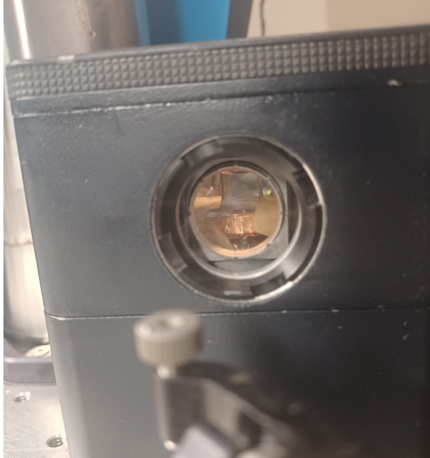
Figure 6.2: A 10\text{mm} \times 10\text{mm} \times 9\text{mm} sample of 0.01\% \text{ Tm}^{3+} : \text{LiNbO}_3 mounted in a Montana Instruments closed cycle cryostat
