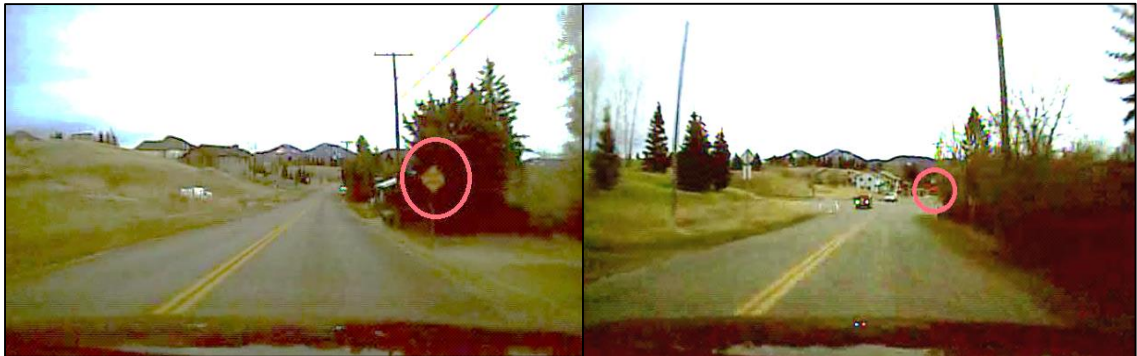
Figure 6: Curved stop ahead on-road scenario: left - “Stop Ahead” warning sign and right- “Stop Sign” obscured by roadside vegetation
