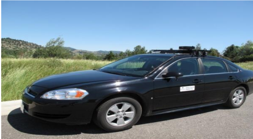
Figure 1: Instrumented Impala with three scene cameras mounted on the top
