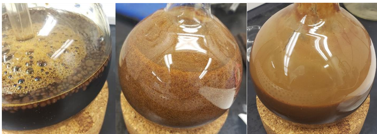
Figure 41. Start of precipitation forming globular lignin particles (left panel), during precipitation significant foaming observed (middle panel), and final acidified black liquor (right panel).
