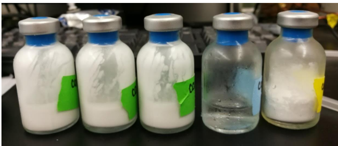
FIGURE 2.5 The experiment vials, filled with calcite in this image. The three vials labeled in green (on the left) are reaction vials with pulverized sample and water. The vial labeled in blue (second from right) is a water-only control. The vial labeled in yellow (right) is a dry sample-only control. Vials are sealed with butyl rubber stoppers and crimp sealed.
