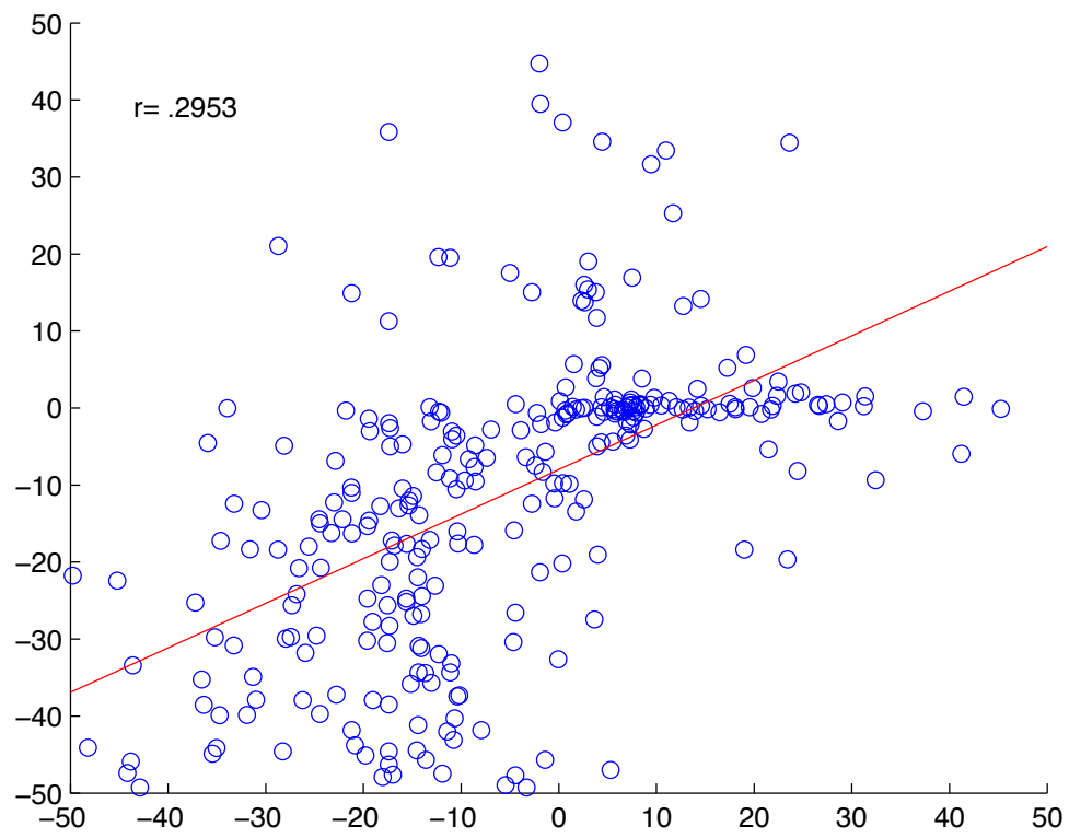
Figure 27: Scatter plot of measured and modeled H with a diabatic correction factor for unstable and stable atmospheric conditions.
