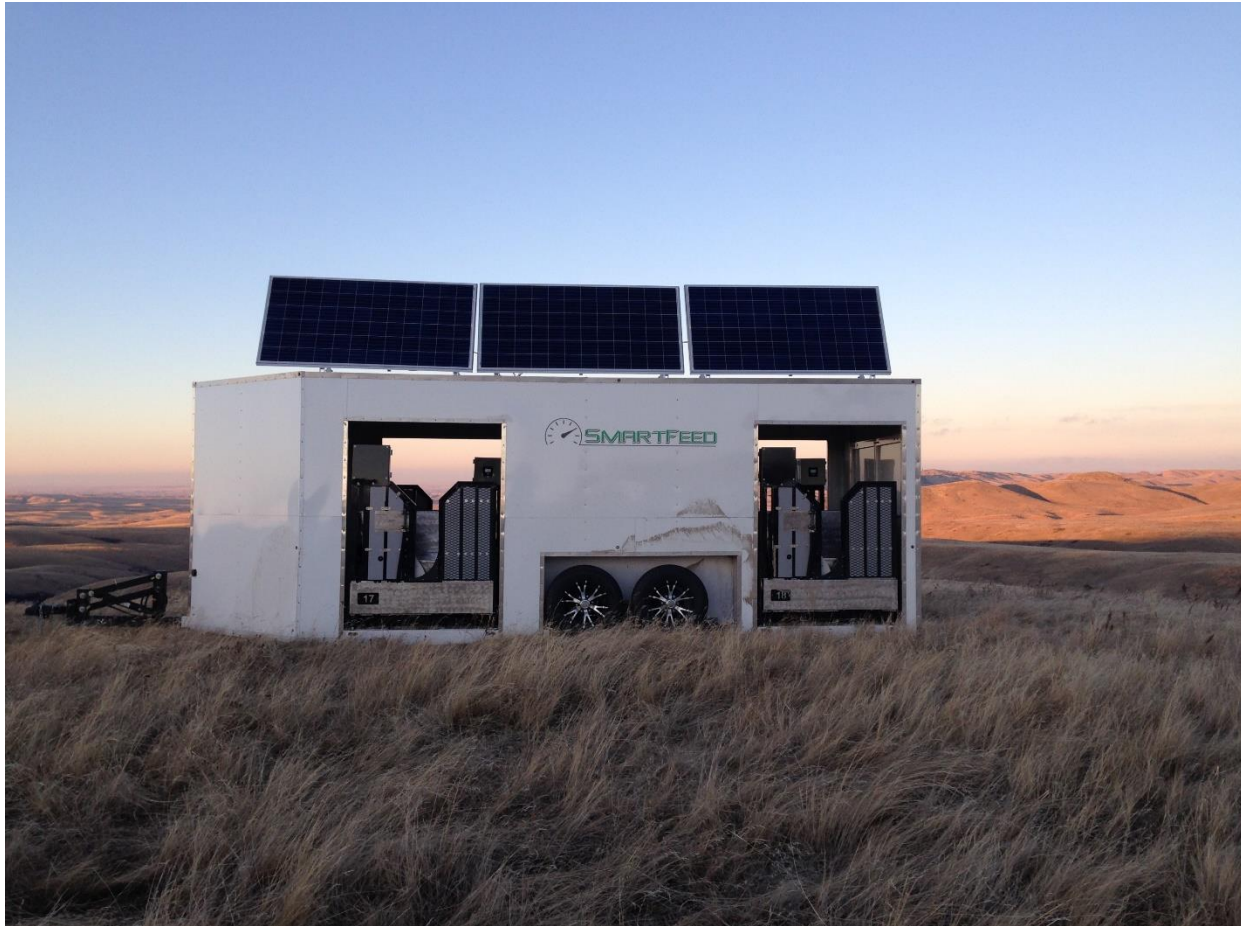
Figure 1. SmartFeed Pro (C-Lock Inc., Rapid City, SD USA) Feed Unit Trailer. Trailer has four feeding stations with two feeders randomly assigned to each treatment supplement.
