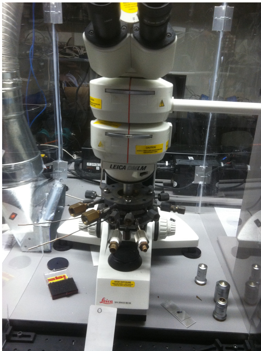
Figure B.2: SAwCER assembled and placed on the microscope stage.
