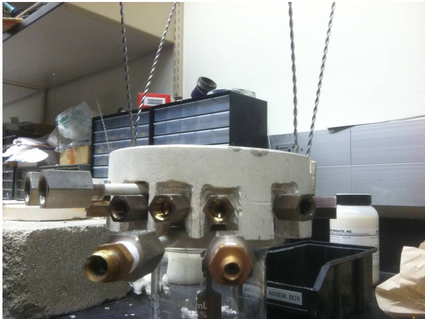
Figure B.5: SAWCER assembled with an inner and outer furnace. Side view.
