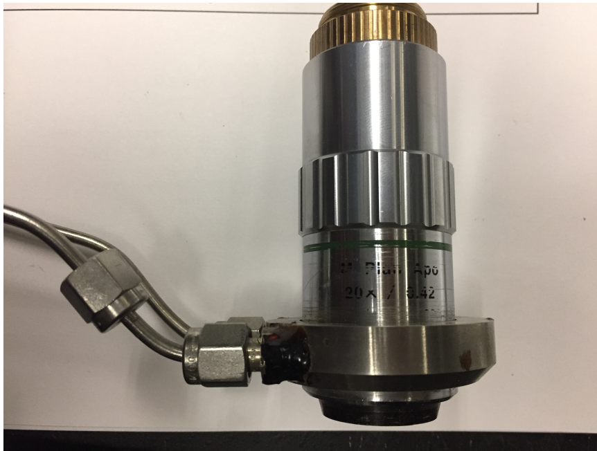
Figure B.6: Objective cooler mounted to the objective.
