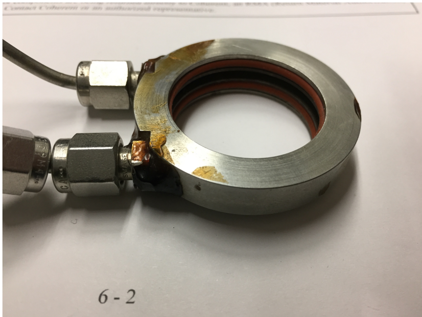
Figure B.7: Objective cooler showing seals.
