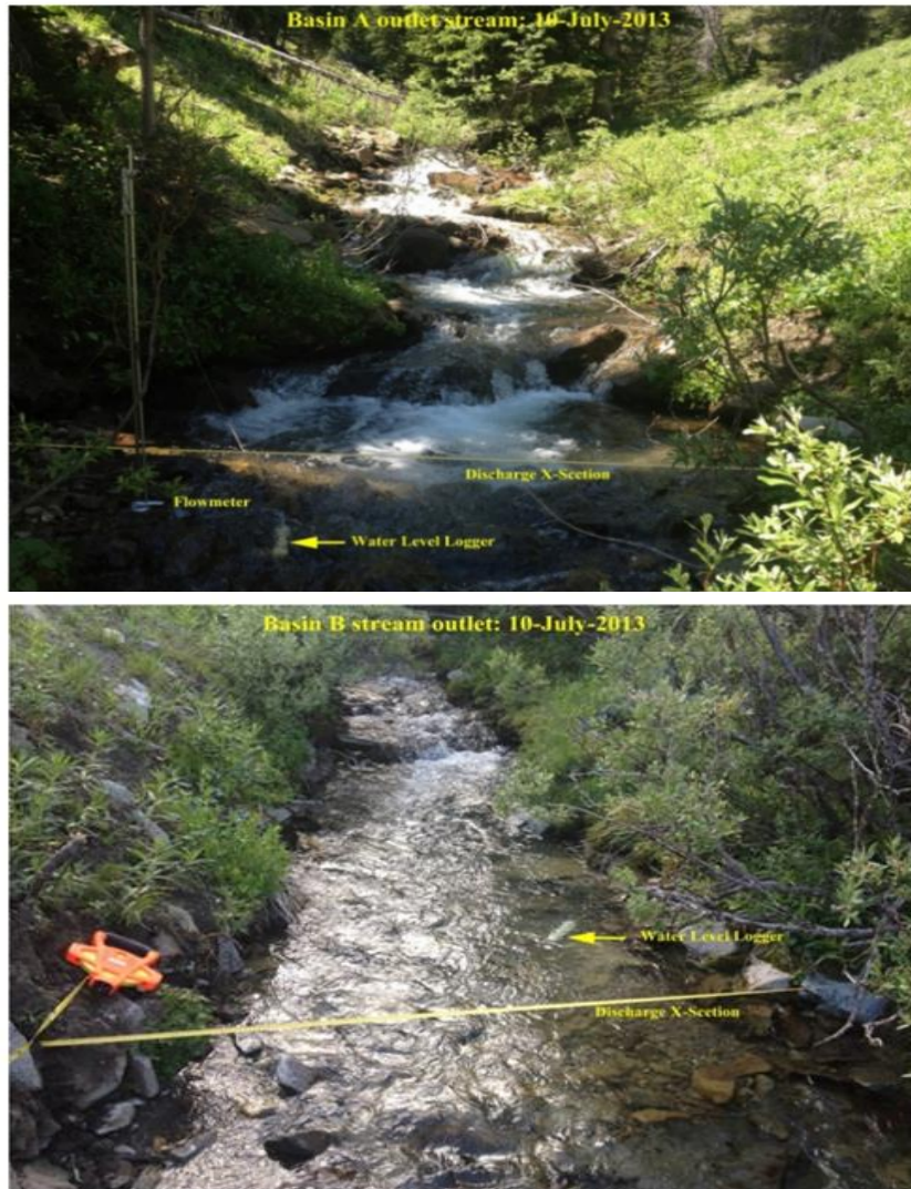
Figure 31. Photos of each stream discharge measurement site on July 10, 2013, showing the water level loggers in relation to the stream cross section where velocity measurements were taken.
