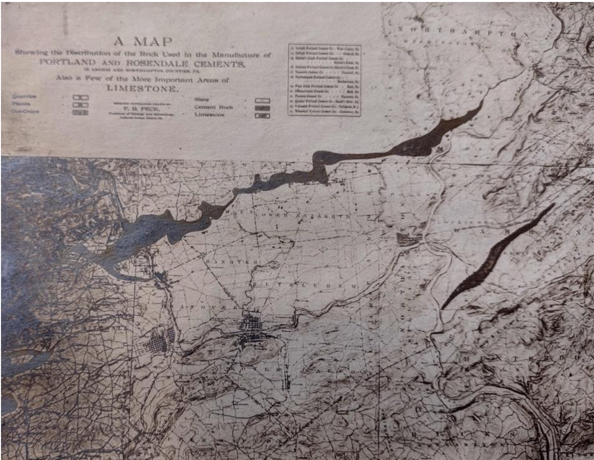
Figure 1.4. Uhler and Atkinson’s thesis also included a copy of this map that their advisor, the geologist F.B. Peck, likely produced for the State of Pennsylvania. Comparison with Figure 1.3 reveals how closely the cement plants followed a regional layer of rock now known as the Jacksonburg Formation. Peck calls this “the rock used in the manufacture of Portland and Rosendale cements,” the latter being a common synonym for natural cement, derived from the Hudson Valley location that produced so much of that material into the late 1800s. The three major Lehigh Valley cities are visible, West to East: Allentown; Bethlehem, with Lehigh University in South Bethlehem; and Easton, with Lafayette College. Image courtesy of Special Collections & College Archives of Lafayette College.
