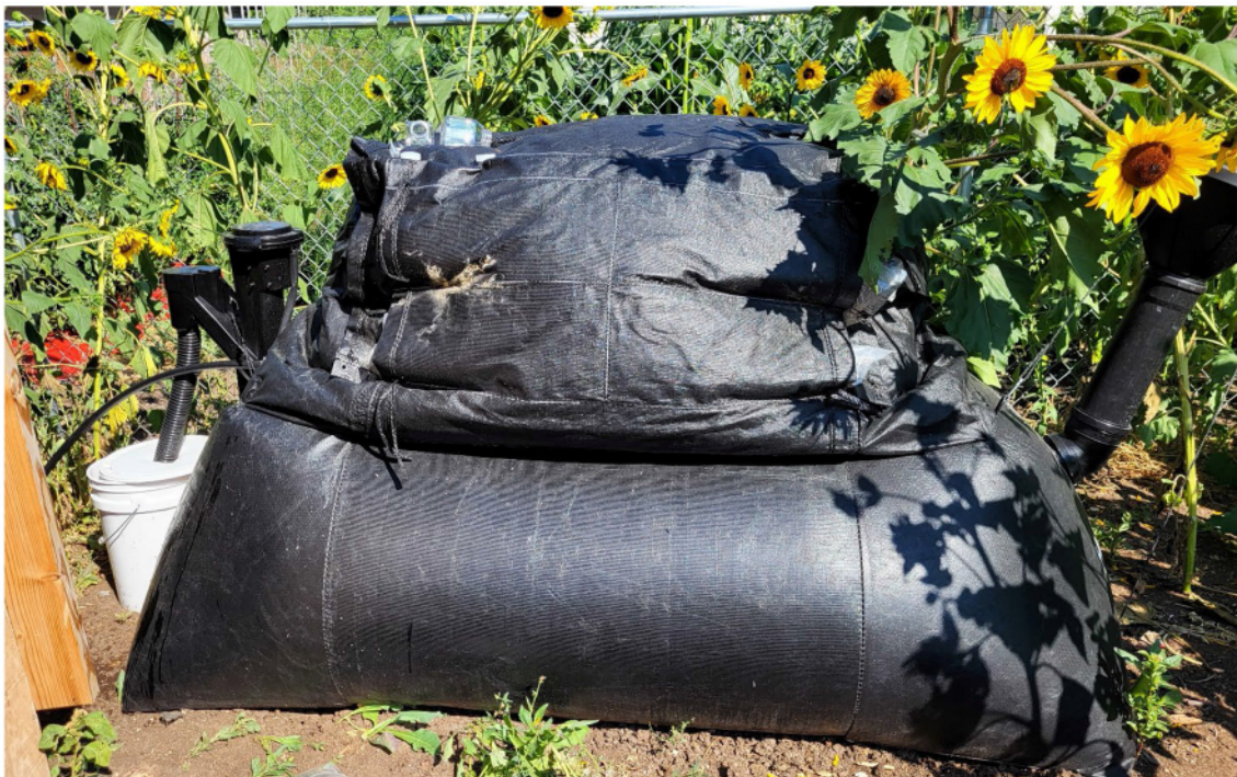
FIGURE 1 Home Biogas digester model in one household's backyard.
