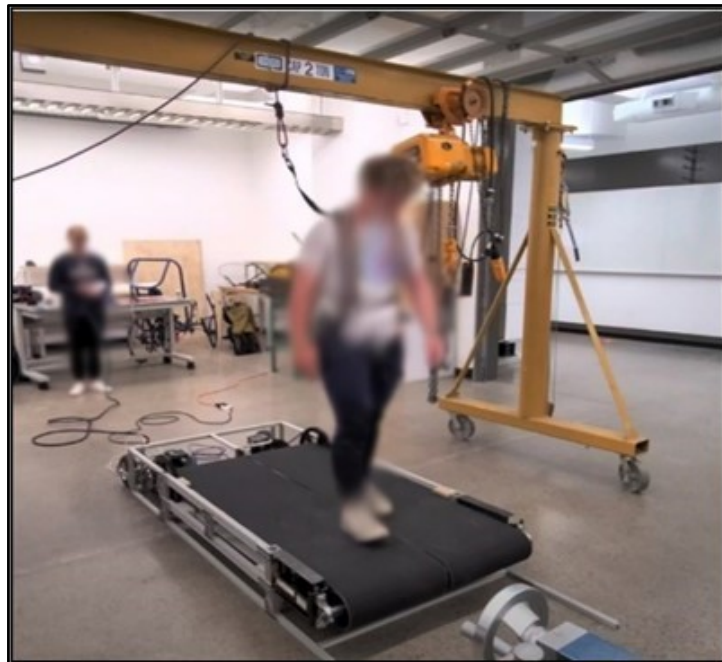
Figure 43. Setup for the Human Test. An undergraduate research assistant stood on the treadmill and was prevented from falling via a climbing harness attached to an overhead crane.
