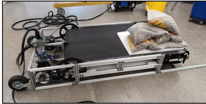
Figure 42. Human Analog Test. Six bags of gravel were placed on the treadmill to determine if the device would be safe to use under maximum load.
