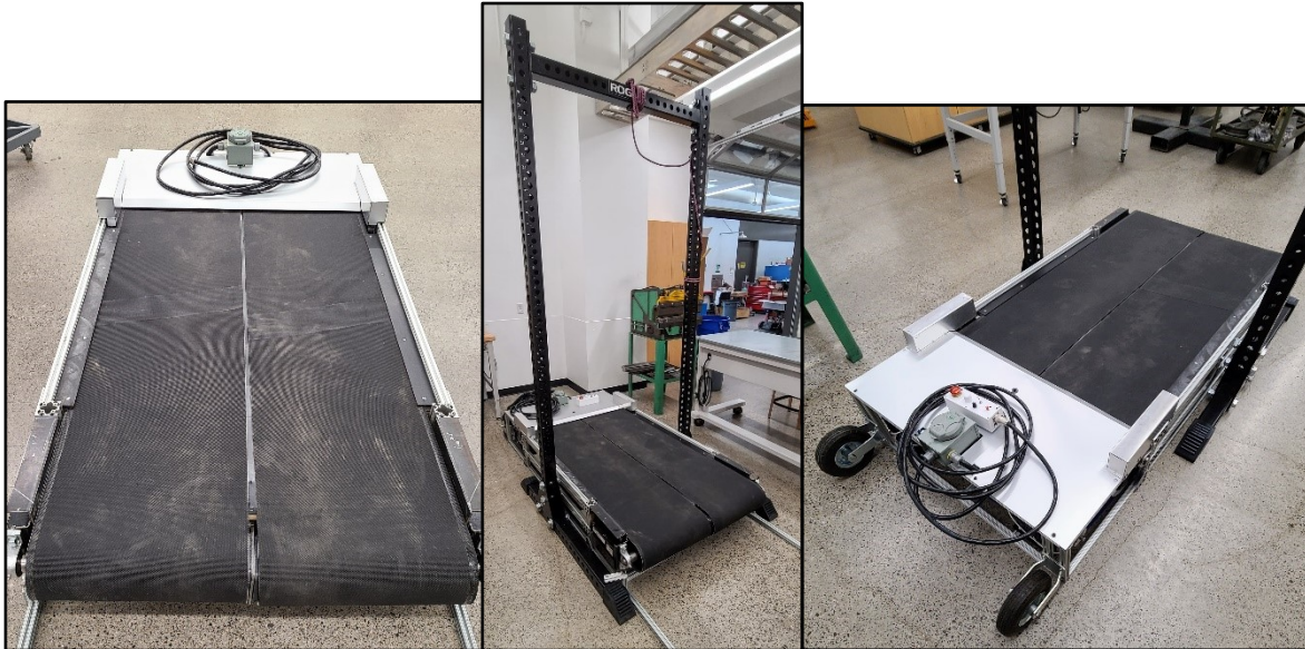
Figure 4. Images of Completed Treadmill. The black frame shown in the middle and right pictures was used to prevent user injury while the treadmill was in use during the clinical trial. This was accomplished via a climbing harness attached to the frame.
