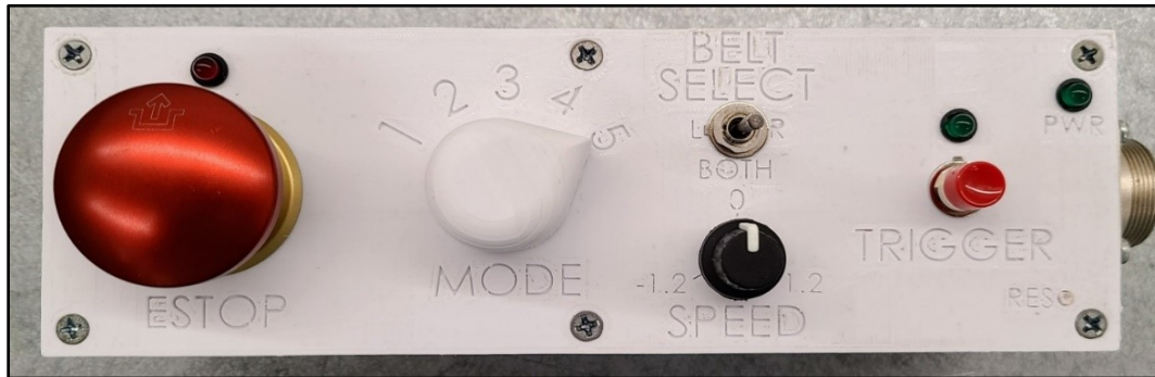
Figure 7. Final Configuration of the Controller Module. Top-down view showing the buttons, switches, and indicator lights used to control the treadmill.
