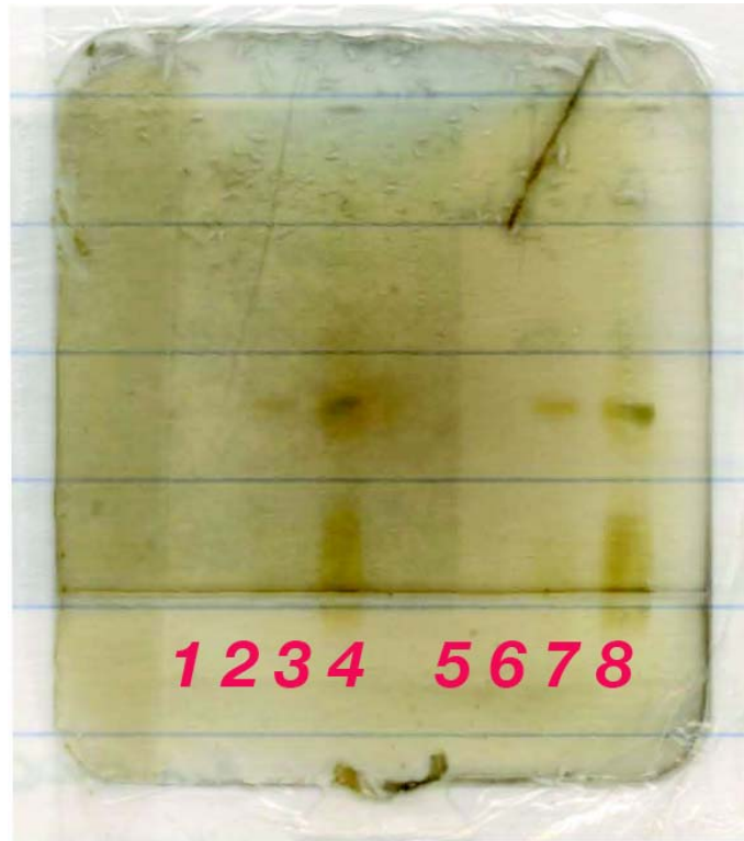
Figure A.4 - Phasta gel showing the effects of filtration upon protein levels run with BSA. In lanes one through four the protein was pushed a 0.22 \mu\text{m} filter and in lanes five through eight the protein is not processed in any way. From lane one to four the concentration of BSA rises from 100 ng, to 1 \mu\text{g} , 10 \mu\text{g} , and 100 \mu\text{g} consecutively. In lane five through eight the protein concentration increases in the same manner.
