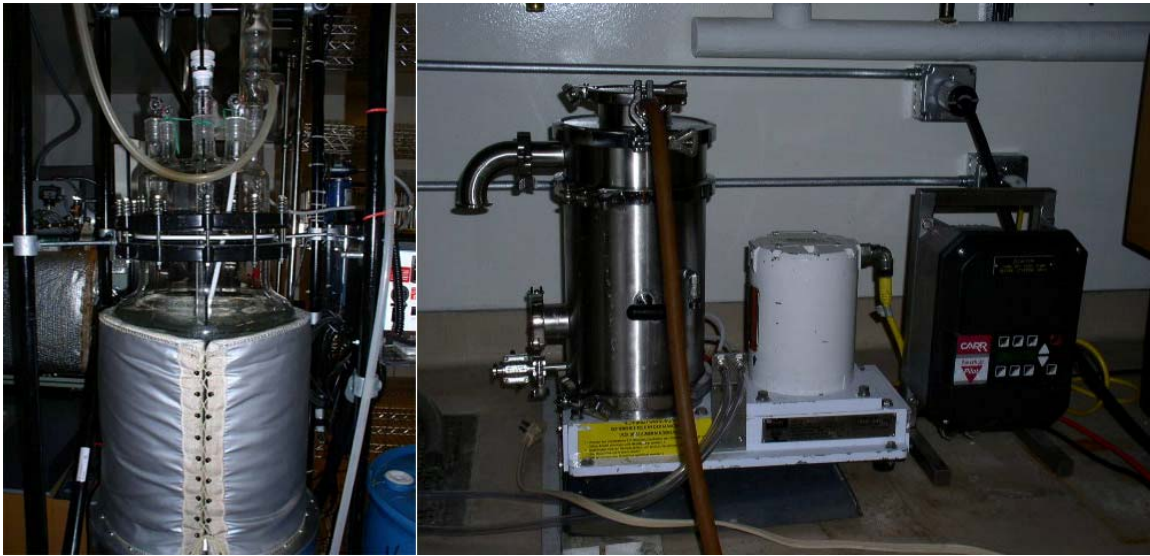
Figure 3.2 - Image of the glass 100 L fermentor (shown with heating element wrapped around) on the left, and the centrifuge filter on the right. A valve is opened at the bottom of the fermentor to run the virus producing culture through the in-line centrifuge when it is ready for processing.
