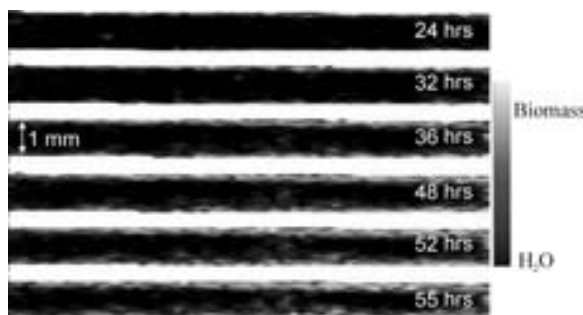
Fig. 5.1.4 Time lapse T_2 maps of biofilm structures as a function of growth. The T_2 maps are collected at different stages in the growth of a biofilm at the time shown after initial inoculation. Light colors indicate water restricted within a biofilm and black is the bulk unrestricted water. Images are acquired in the absence of flow, however the flow direction for growth periods between images is left to right [15].
