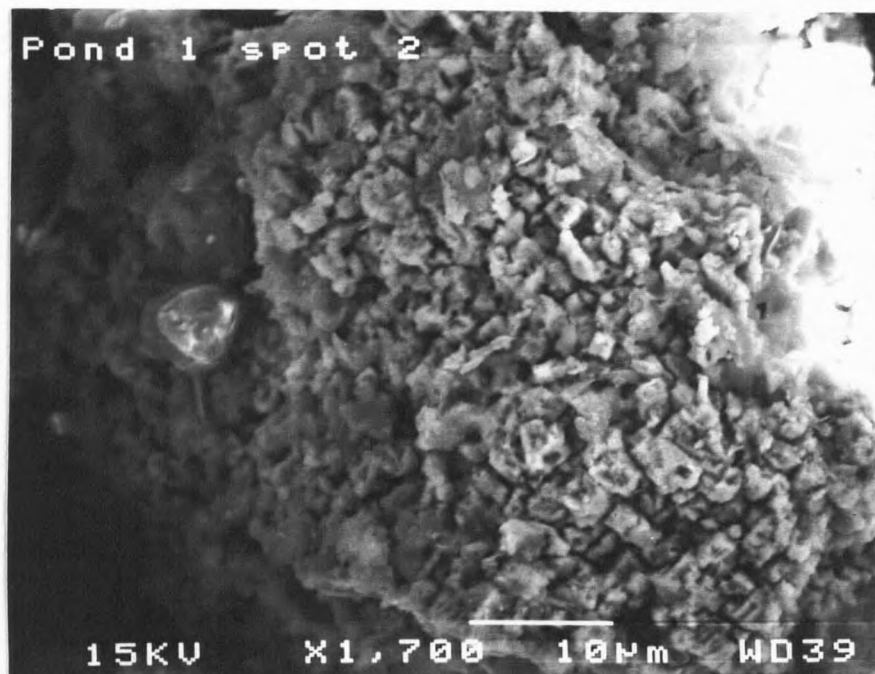
Figure 12. Cu sulfide particle from FW1 sediment. Larger particle is composed of many small Cu sulfide precipitates.
