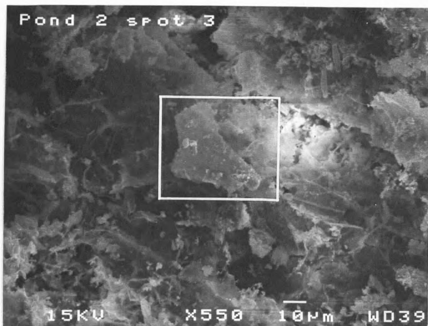
Figure 8. SEM photograph of Zn solid phase from FW2 sediment. The ratio of Zn and Si (Zn:Si = 8.5:5.3 elemental %) suggests that Zn is either coprecipitated with quartz, or that the solid is the Zn silicate mineral willemite ( \text{Zn}_2\text{SiO}_4 ).
