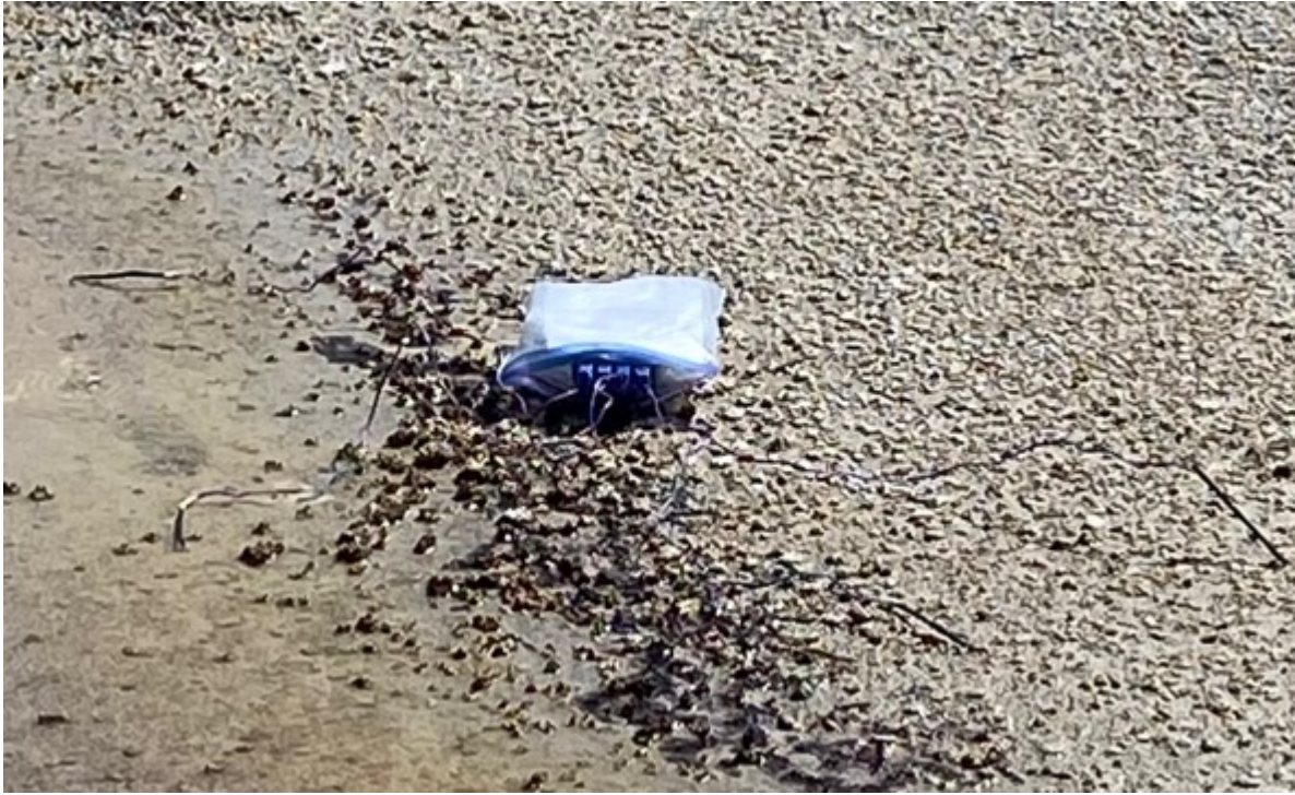
Figure 3. Thermocouple reader/recorder recording temperatures at Dragon Spring. Two thermocouples were positioned near the surface of the water. The other two (not shown) were recording substrate surface temperature.
