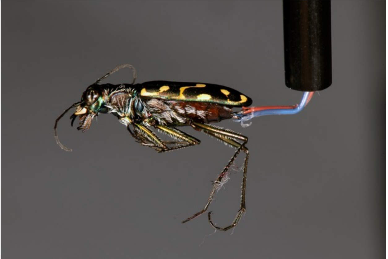
Figure 1: Cicindelidia haemorrhagica adult with a thermocouple inserted into its abdomen in preparation for water bath experiment. Photo by RKD Peterson.
