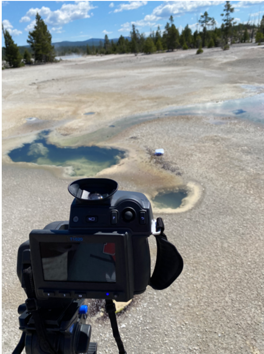
Figure 2. Thermal recording equipment on-site at Dragon Spring. The thermocouple reader/recorder can be seen in the background recording substrate and water temperatures while adult Cicindelidia haemorrhagica traverse the area.
