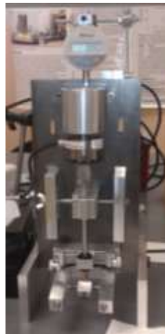
[Figure 11: Vertical Loading System] during testing the cylindrical pot attached directly to the load cell is loaded with vials of steel shot, and the compression distance of the spring is measured via the digital dial indicator at the top.
