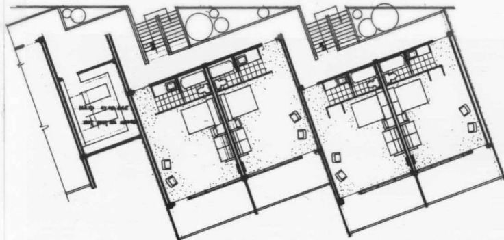
FLOOR PLAN UNIT GROUP 1 (GROUP 2 SAME, ROT 40° CLOCKWISE)
