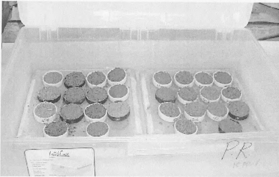
Figure 31. Racks inside plastic containers that hold soils saturated with synthetic waters.
