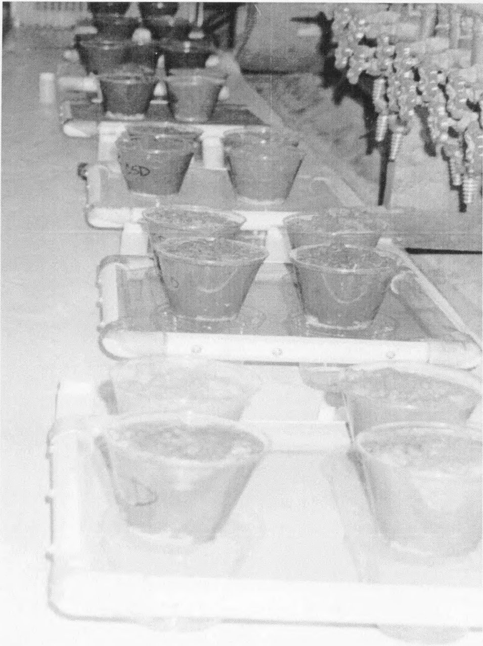
Figure 18. Samples were placed on mesh racks, so that distilled water would leach through the soil. This was the 5X + d treatment.
