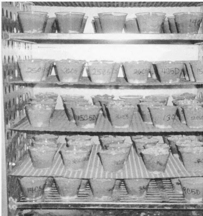
Figure 17. Soil samples were dried to 35^{\circ}\text{C} between wetting regimes.
