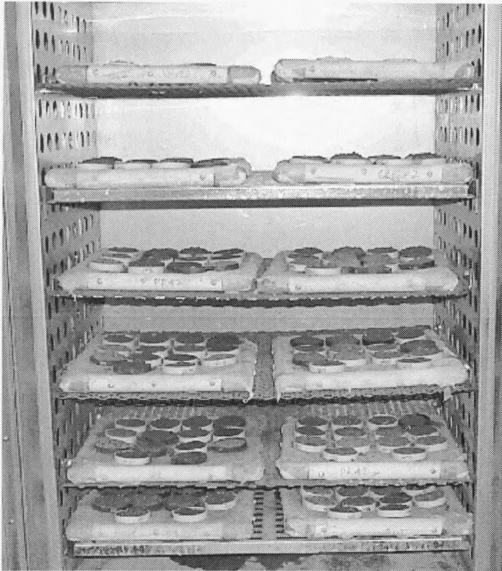
Figure 32. Racks holding soil samples were dried to 35°C between wetting regimes.
