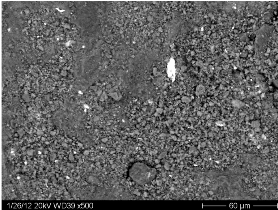
Figure C.1. Back-scattered electron image of surface of individual grain from the 2-4 mm size class of basal melt-out till sediments. Note coverage of significant portions of primary grain surface area with grain fragments.
