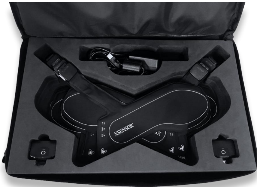
Figure 38. The XSensor Pro Intelligent Insoles used to measure ground contact time and ground reaction force.
