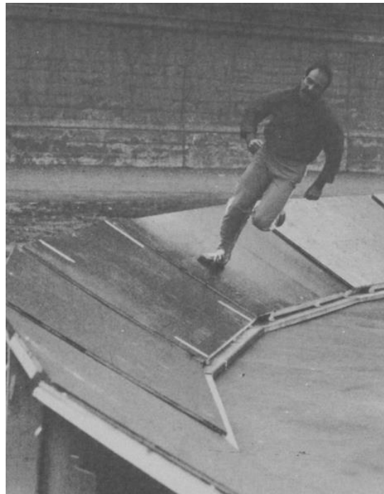
Figure 9. A photograph from one of the oldest studies regarding running on banked tracks. Greene 51 constructed a banked track out of plywood and sections of track surface to show the performance and biomechanical improvements caused by banking a track turn.
