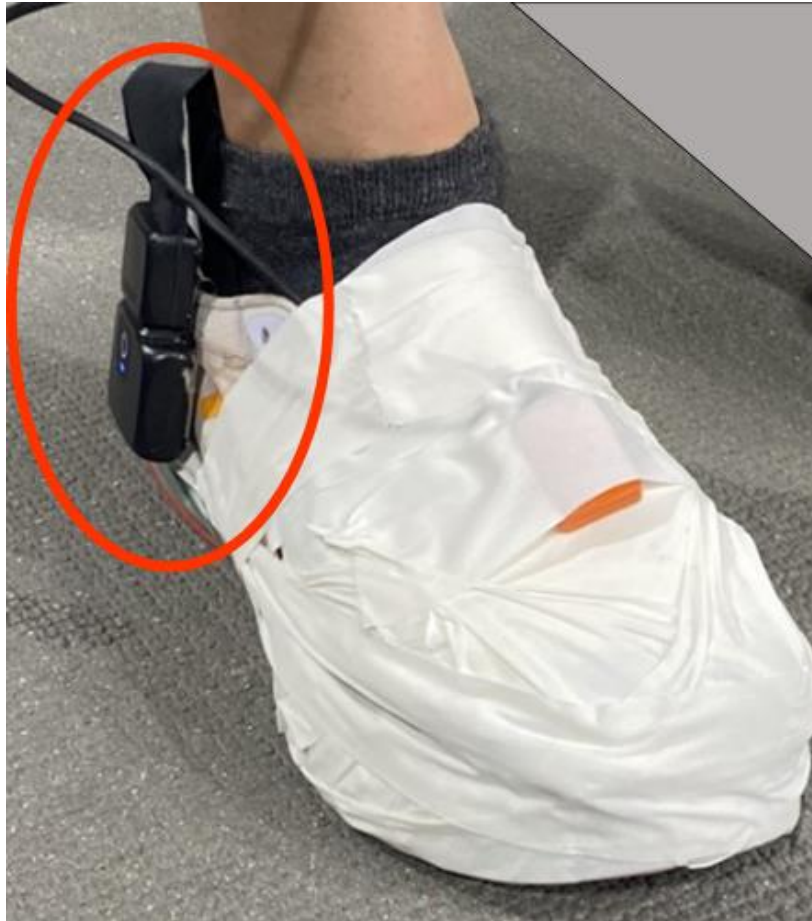
Figure 39. The XSensor pressure insole in an athlete's shoe. The data transmitter and battery clip onto the outside of the shoe.
