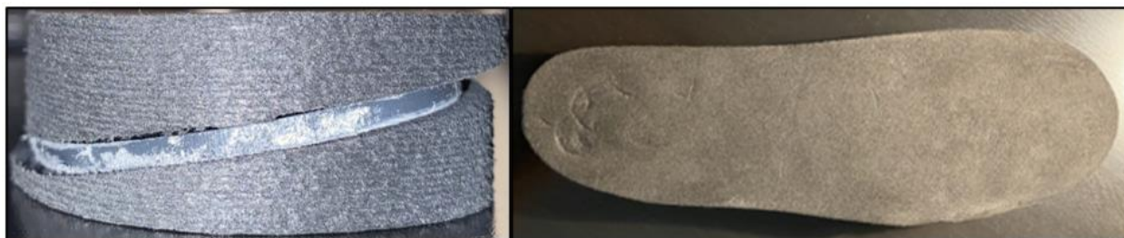
Figure 28. Left to right: front and top view of the angled plate insole prototype.
