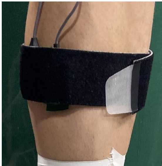
Figure 37. An EMG sensor fixed securely to a gastrocnemius medialis muscle. The sensor was first secured to the skin with double sided tape and then wrapped with an elastic Velcro strap.
