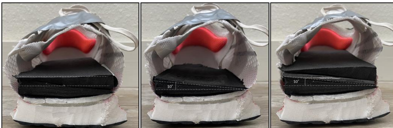
Figure 30. Front view cross-sections of all 3 insoles for the right shoe. From left to right: baseline, wedge, and angled plate insoles. The wedge and angled plate insoles were each compared to the baseline insole.
