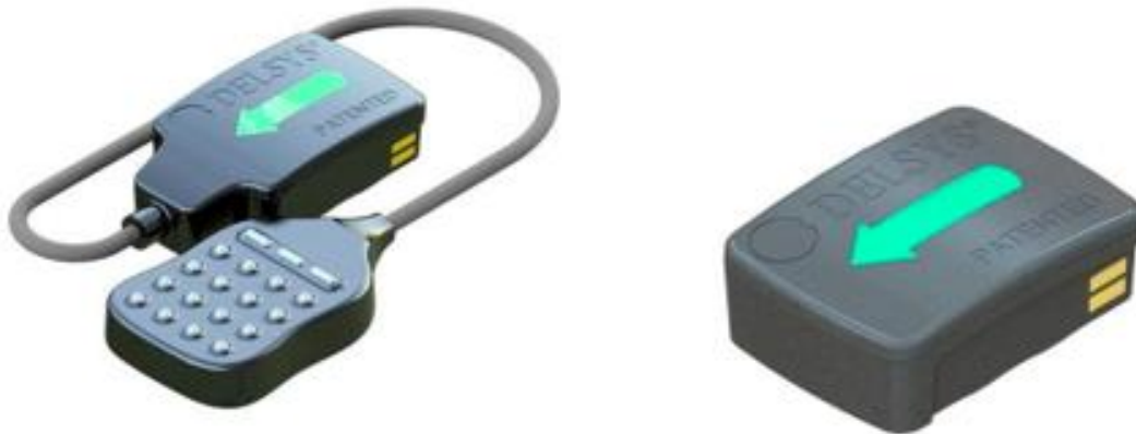
Figure 35. Trigno Maize sensor (left, multi-channel) and Trigno Avanti sensor (right, single channel). The Maize sensors were used on the gastrocnemius medialis, and the Avanti sensors were used on the gluteus medius.
