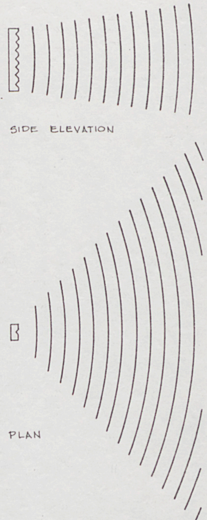
Fig. 53. A line-source or column loud-speaker and its coverage characteristics
