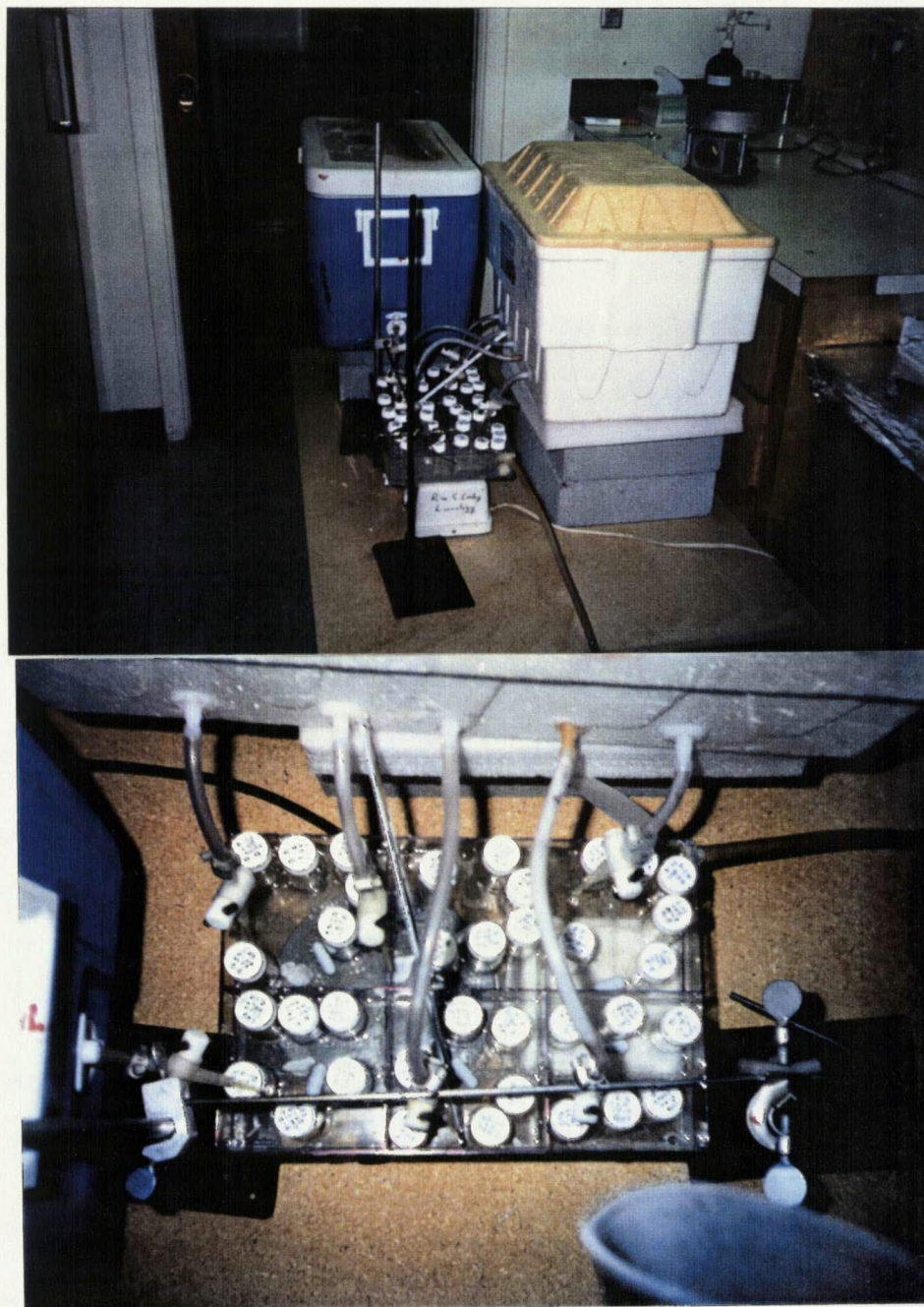
Figure 37. Polythermostat used to assess the temperature response of bacterioplankton.
