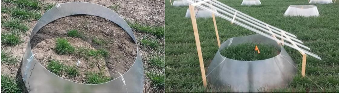
Figure 3.2. Open top chamber (OTC) (left) designed to generate a warming effect of \sim 2^{\circ}\text{C} on the plot, while receiving ambient moisture levels. Rain out shelter with open top chamber (ROS+OTC) (right) intended to reduce \sim 50\% of precipitation from entering the plot as well as facilitate warming.
