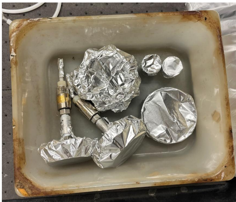
Figure G6. Autoclave tray with reactor parts foiled for sterilization. Before autoclaving, a sheet of foil should be placed over the entire tray.
