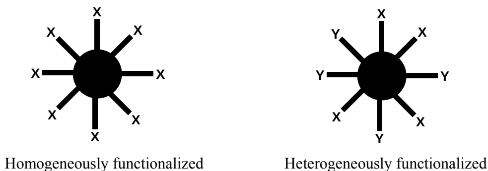
Figure 1.5 Schematic representations of homogeneously and random heterogeneously functionalized dendrimers
