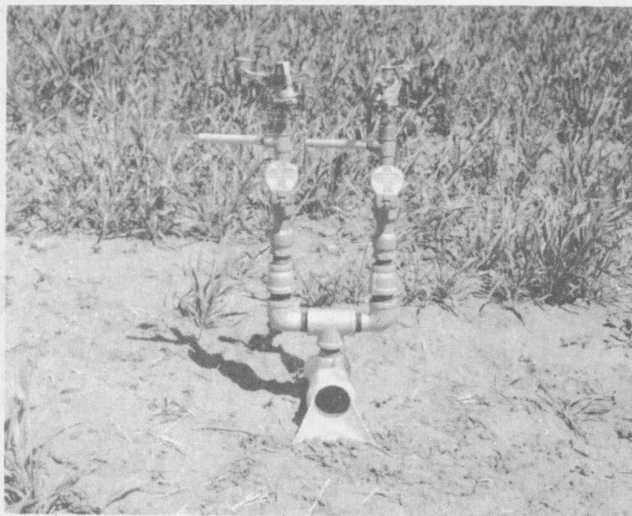
Figure 3. Two-inch coupler with double valve riser.
