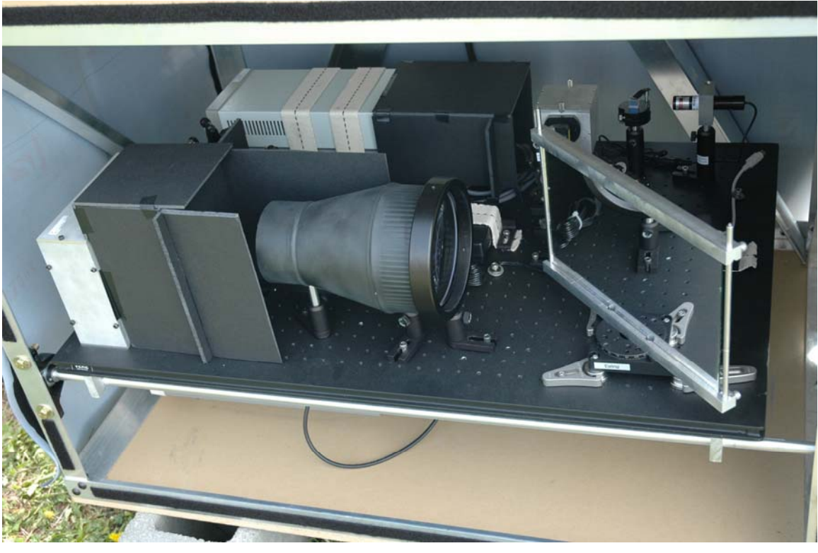
Figure 2. Photo of the Wingbeat Modulation Detector (photo by Joseph A. Shaw).
