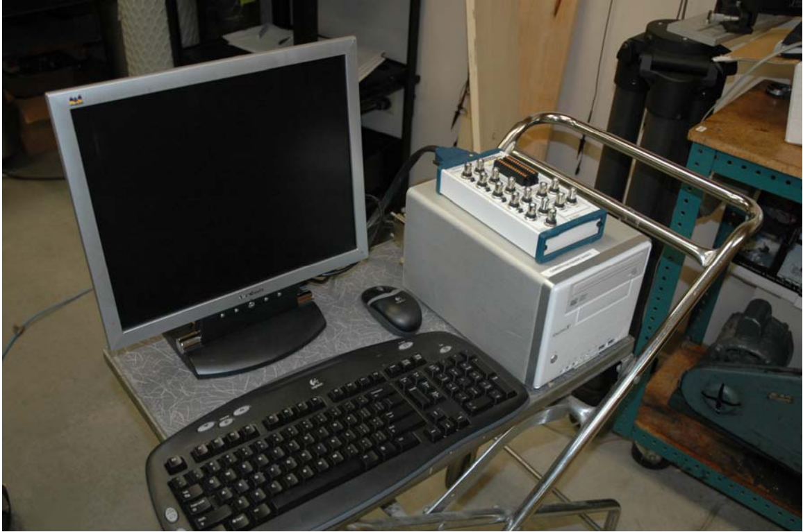
Figure 5. I/O block for the A/D card and computer.
