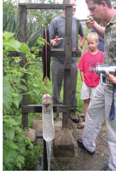
Fig 4.5 Local materials (twine, simple rubber stops, metal pieces) make up this hand cranked pump. The twine has knots in it with rubber stops tied to them, which are pushed into a pipe to trap air. This creates enough pressure in a cistern to push water up into the spigot.
