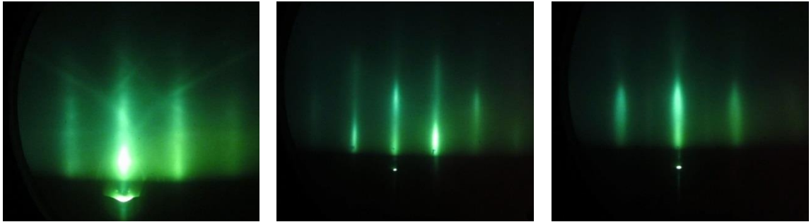
Figure 4-2 RHEED images (LEFT) from the bare MgO(001) substrate taken along the \langle 100 \rangle direction, (CENTER) for a 20 nm pure Fe film on MgO(001) along the \langle 100 \rangle direction of the MgO substrate, and (RIGHT) for a 20nm Fe 80 Mn 20 film on MgO(001) along the \langle 100 \rangle
